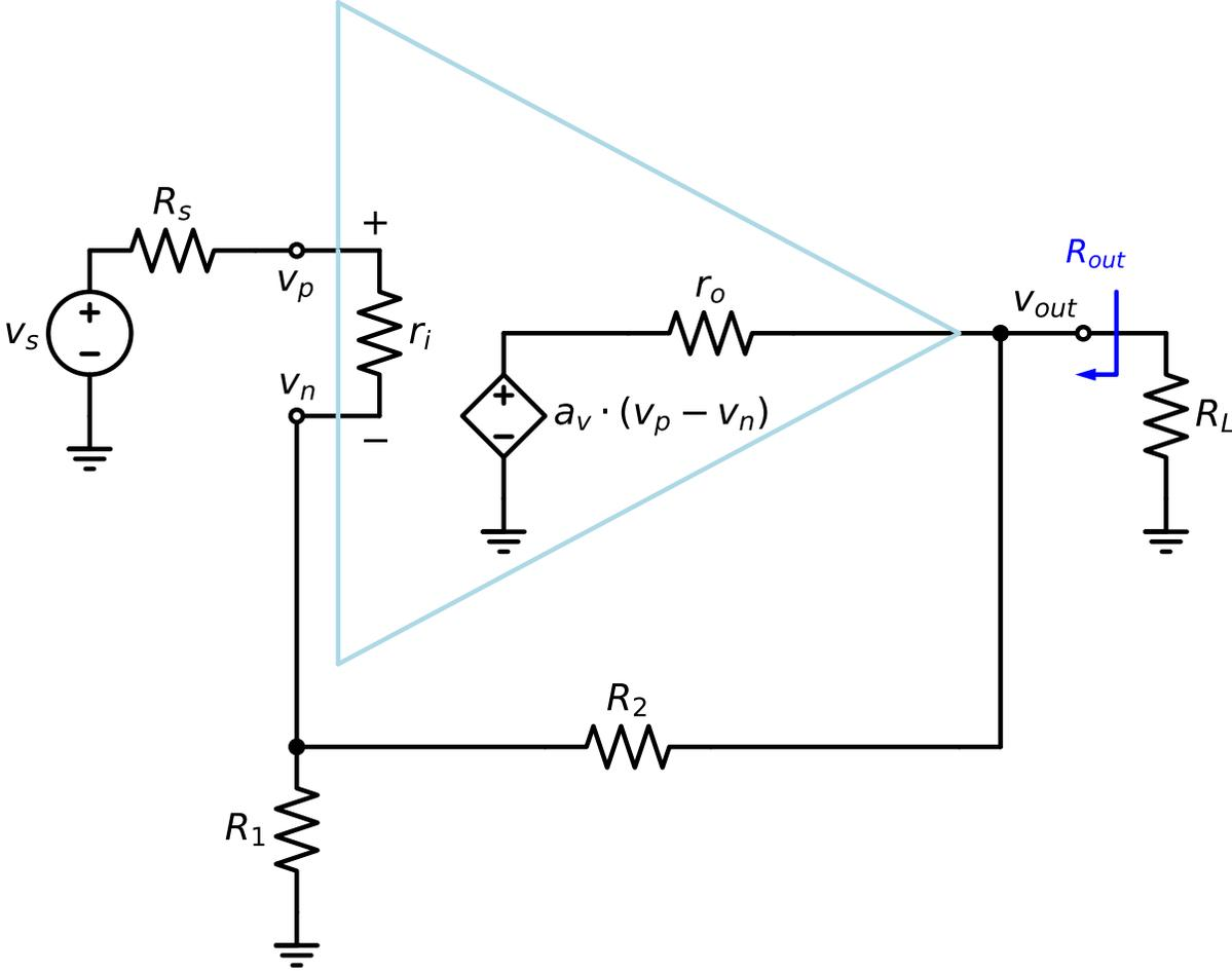
Figure 7.53.: Output resistance of non-inverting op amp circuit
