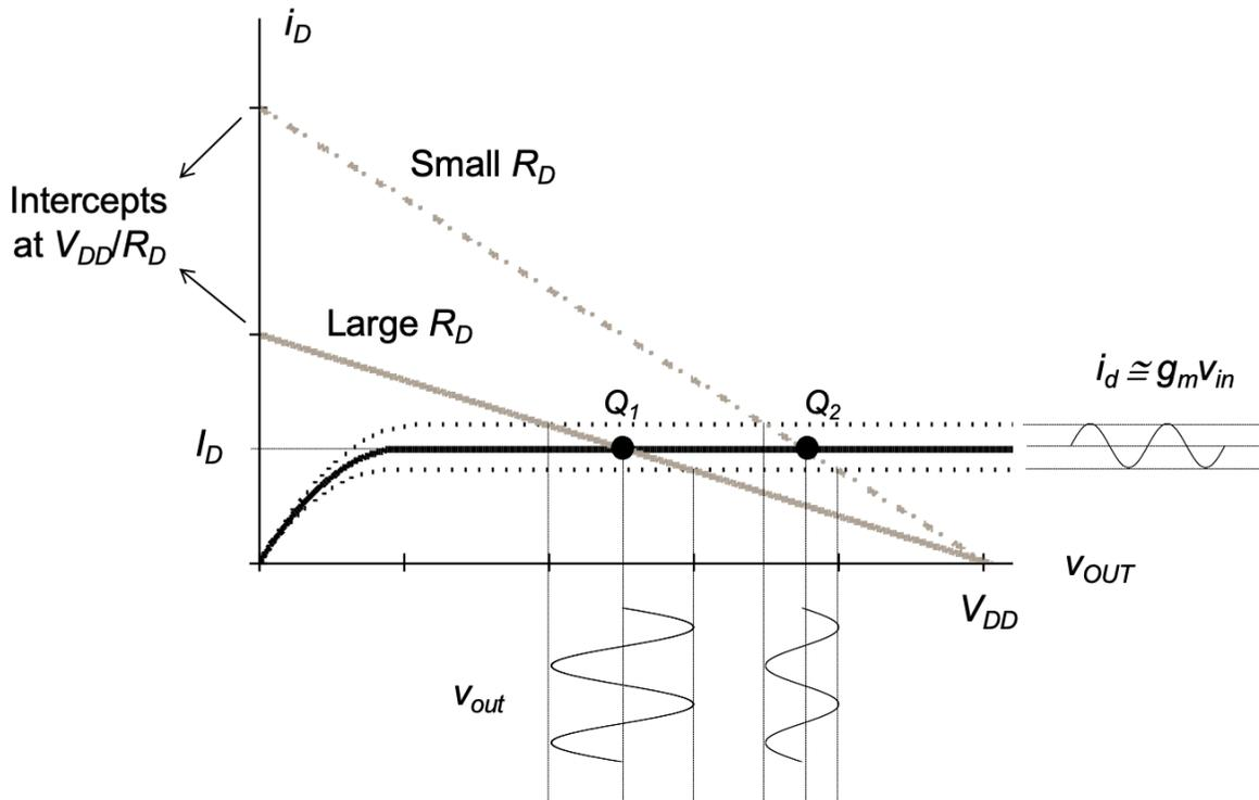
Figure 2.18.: Amplifier load lines for large and small values of  $R_D$ .
