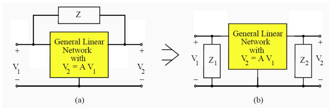
Figure 3.17.: Illustration of the Miller theorem.
