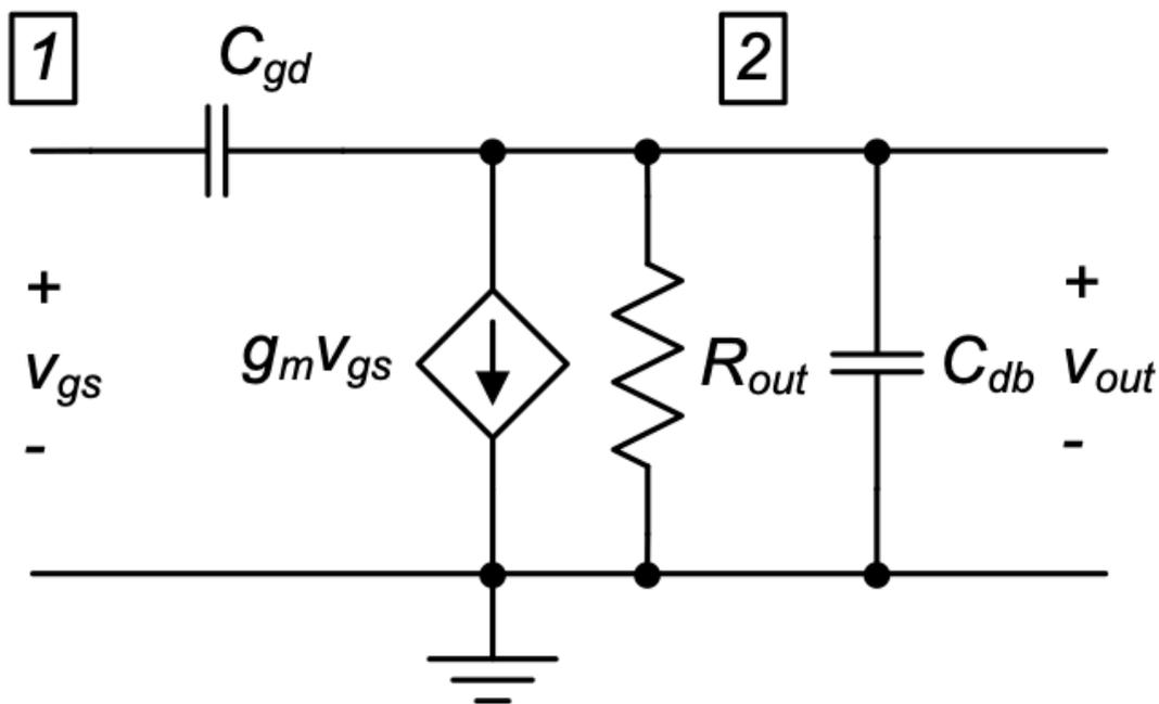
Figure 3.19.: Circuit to analyze the voltage gain across  $C_{gd}$ .
