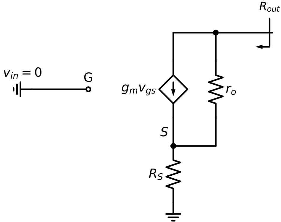
Figure 7.74.: Small signal model to find the output resistance
