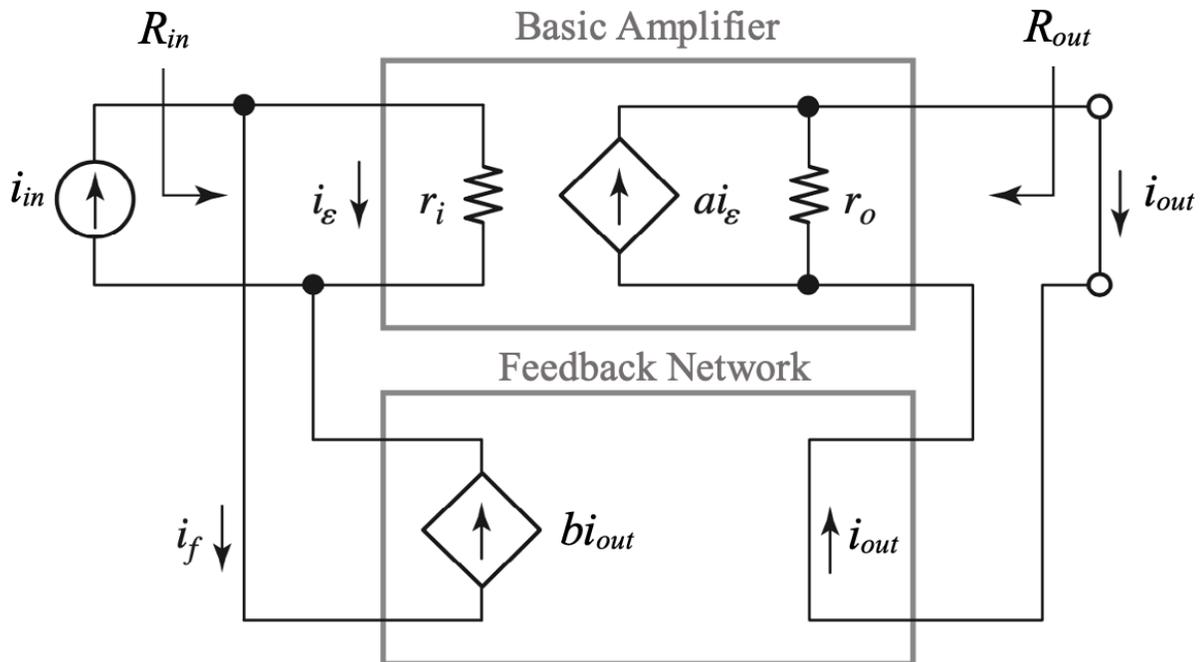
Figure 7.14.: The shunt-series configuration or current amplifier (Franco 2015)
