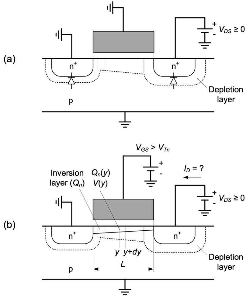
Figure 2.2.: (a) n-channel MOSFET with  $V_{GS} = 0$ , (b)  $V_{GS} > V_{Tn}$ ,
