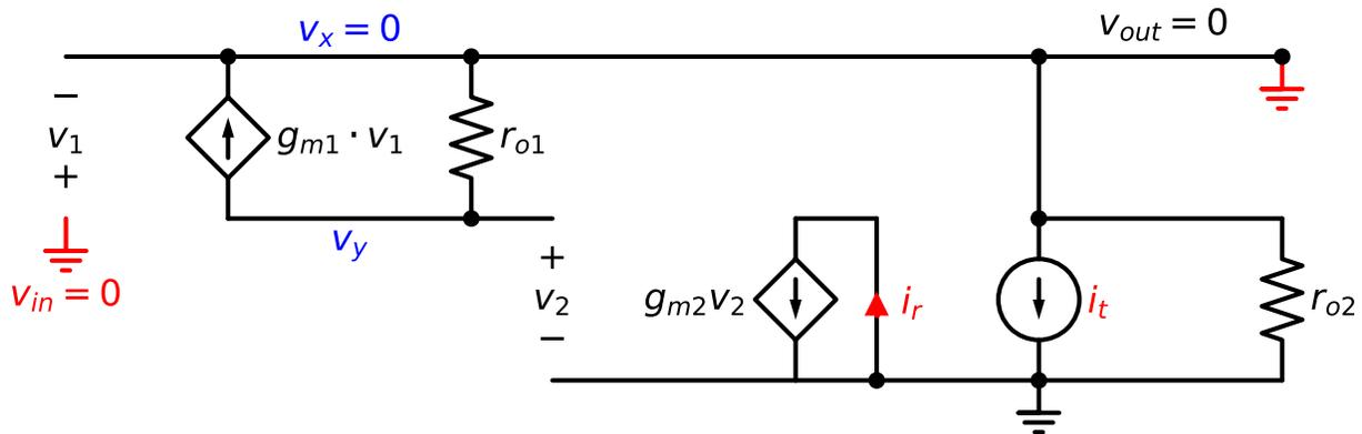
Figure 7.61.: Return Ratio for  $g_{m2}$  with the output port shorted
