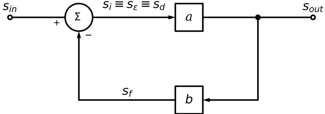
Figure 7.2.: Block diagram of a negative feedback system.
