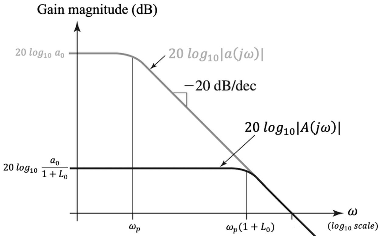
Figure 7.9.: Gain magnitude vs. frequency for the basic amplifier and the feedback amplifier
