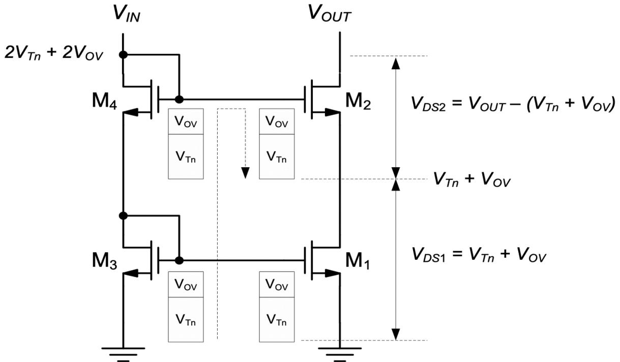
Figure 5.18.: Analysis of the compliance voltage in the basic cascode current mirror.
