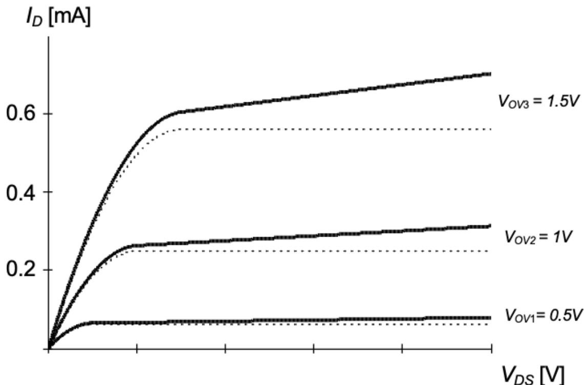
Figure 2.22.: Realistic n-channel I-V plots, incorporating the dependence of saturation drain current on  $V_{DS}$ . (solid lines), along with the first-order model assumed previously (dotted lines). Parameters:  $W = 20 \mu m$ ,  $L = 2 \mu m$ .
