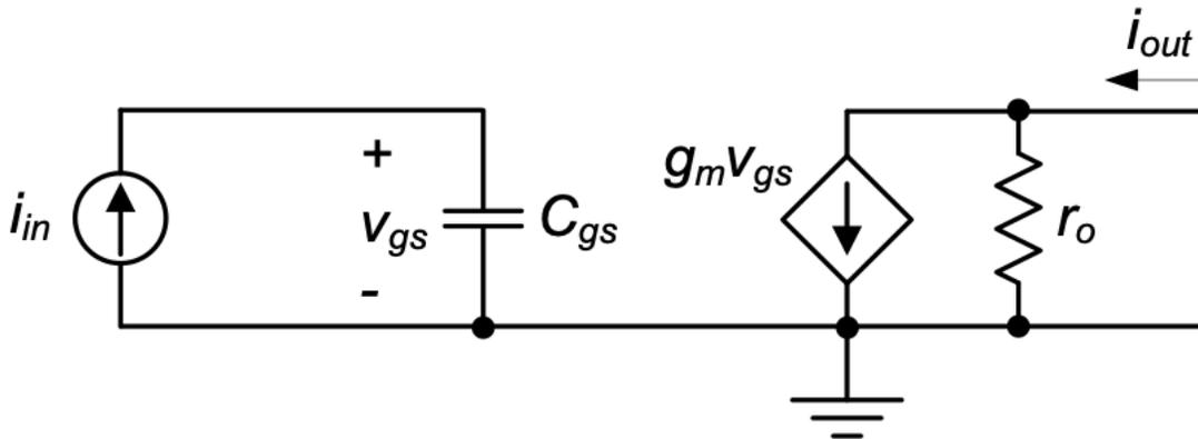
Figure 3.11.: Small-signal circuit model for finding the MOSFET's transit frequency.
