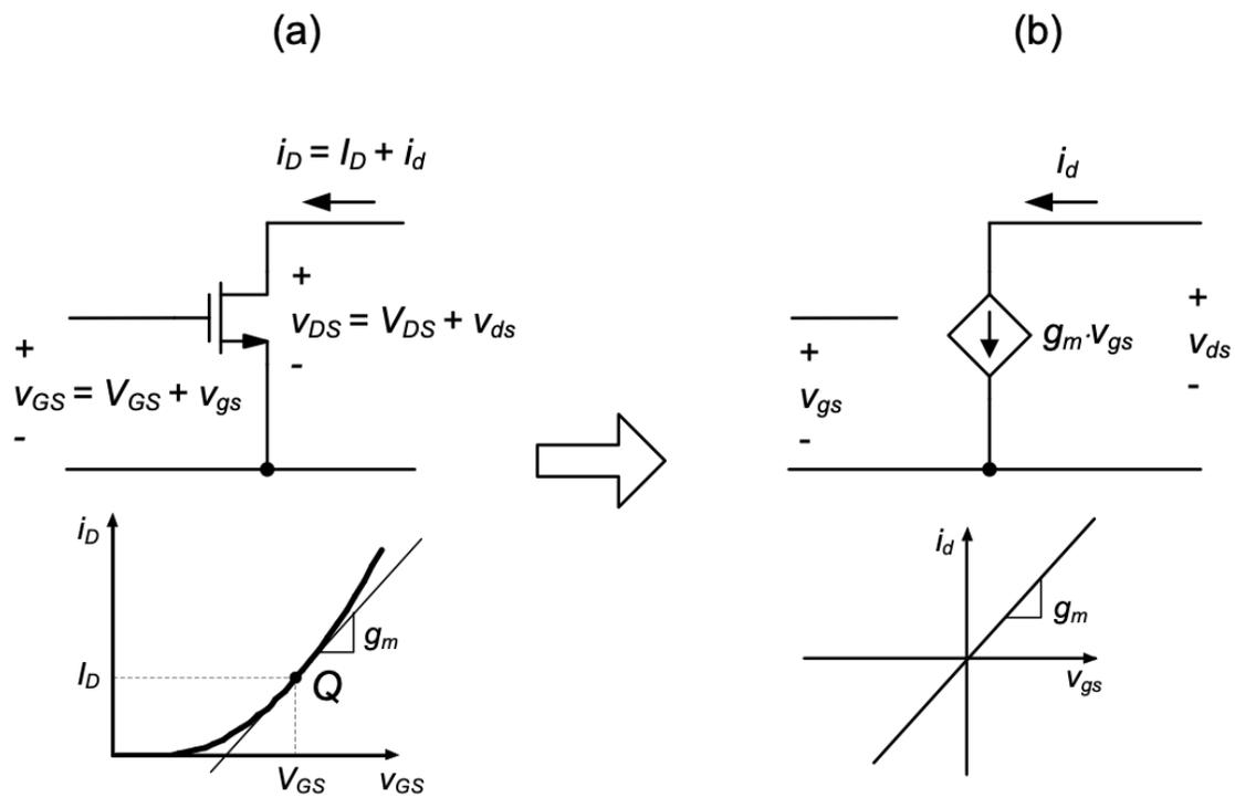
Figure 2.13.: (a) Large-signal transfer characteristic of an n-channel MOSFET in the saturation region. (b) Small-signal transconductance ( $g_m$ ) at the operating point.
