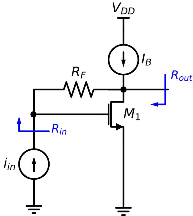
Figure 7.63.: Shunt-shunt stage (Transimpedance Amplifier)
