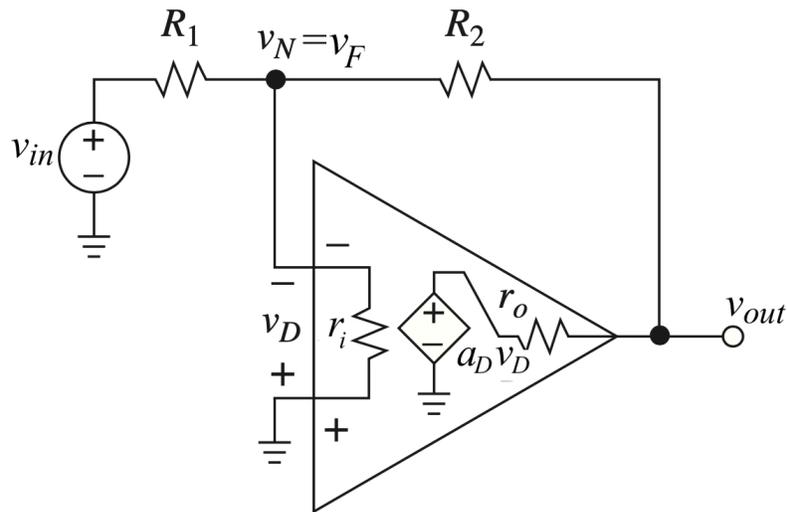
Figure 7.19.: Inverting op amp amplifier. (Franco 2015)}
