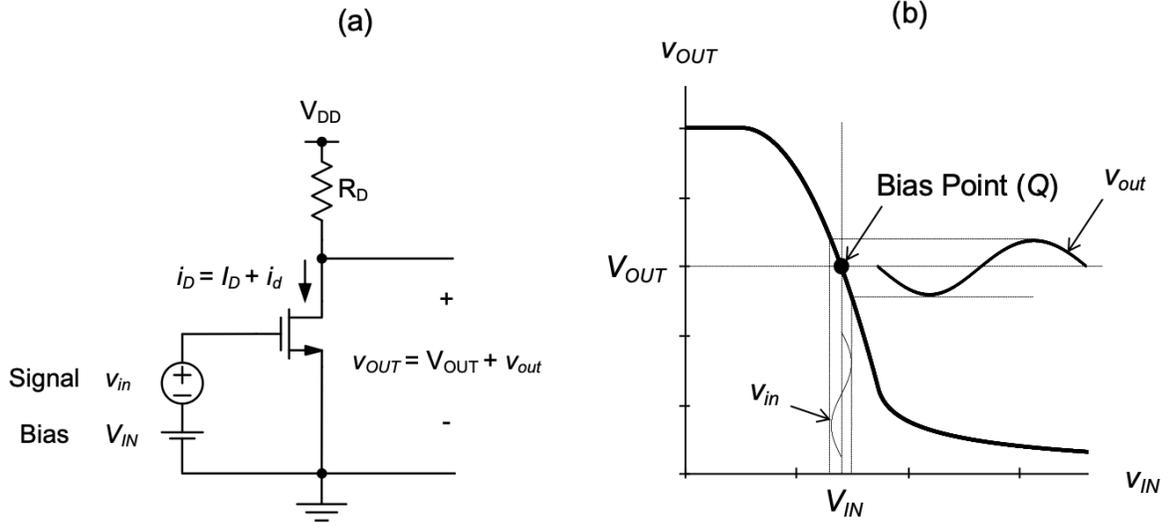
Figure 2.10.: (a) CS amplifier with input bias.(b) Transfer characteristic showing the bias point.
