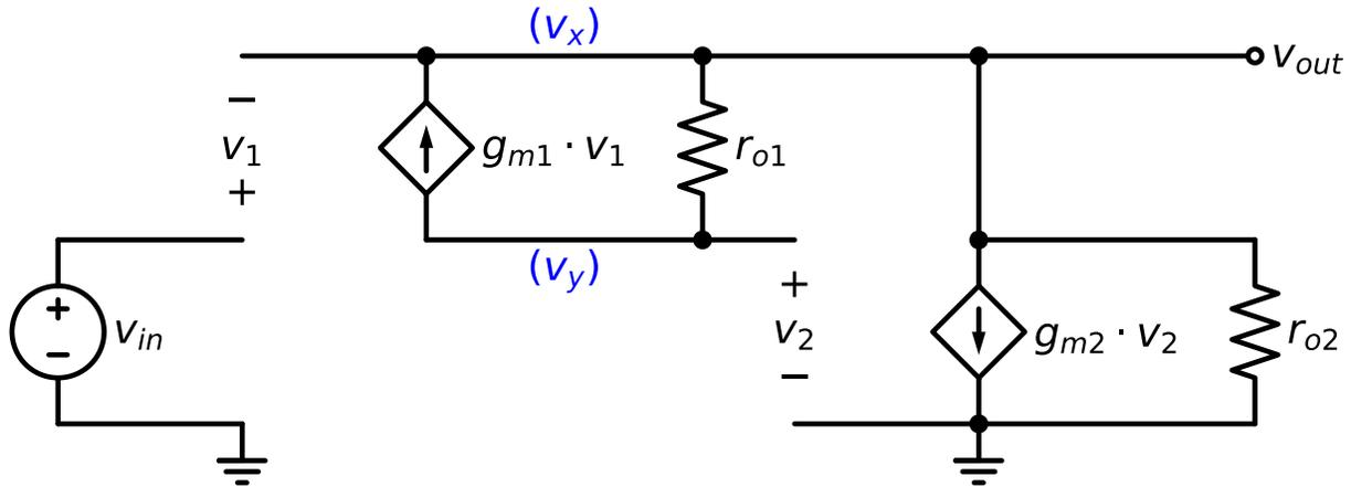
Figure 7.60.: Small-signal model of the super-source follower
