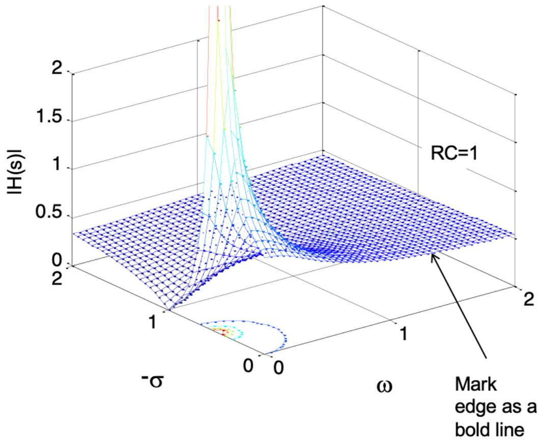
Figure 3.5.: 3-D plot of the magnitude of Equation 3.5, evaluated for  $s = \sigma + j\omega$ .
