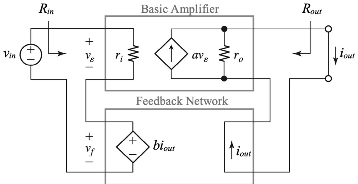
Figure 7.13.: The ideal series-series configuration or transconductance amplifier (Franco 2015)
