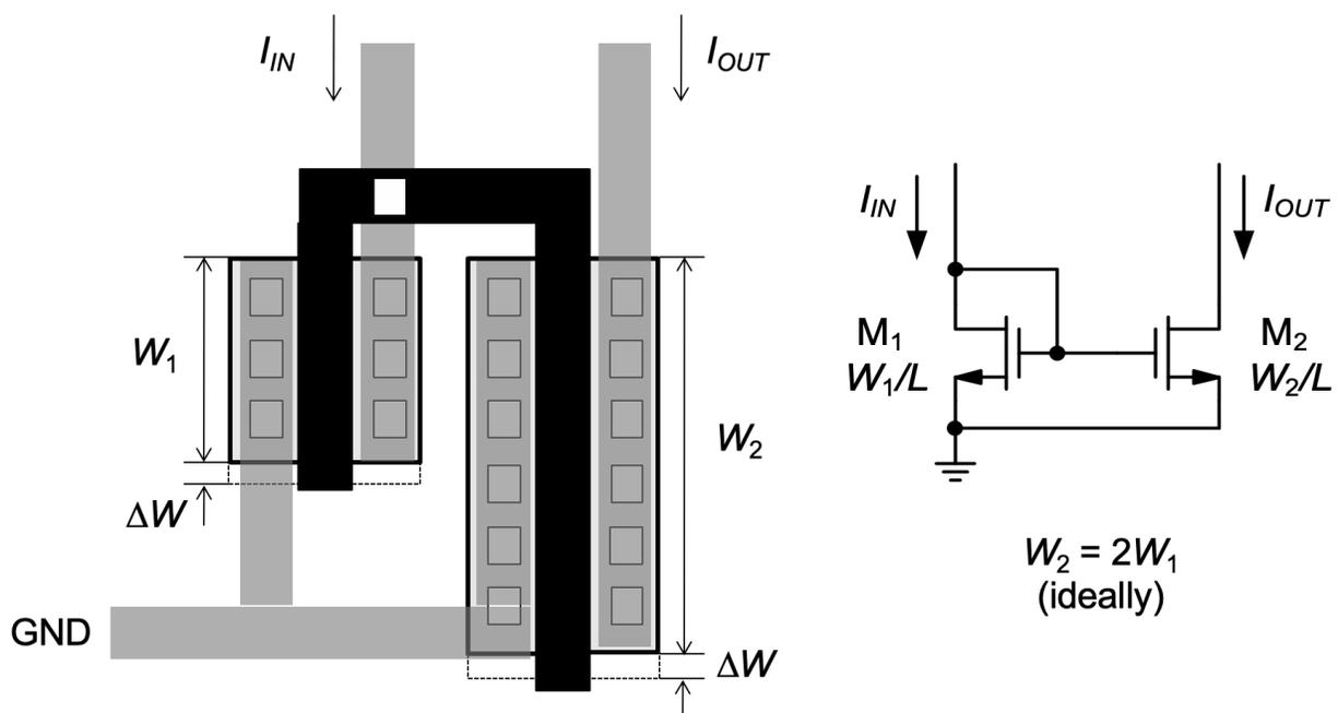
Figure 5.5.: Layout of a current mirror with a desired current ratio of two.
