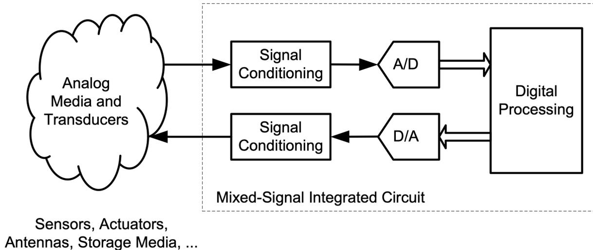
Figure 1.1.: Block diagram of a mixed-signal system.
