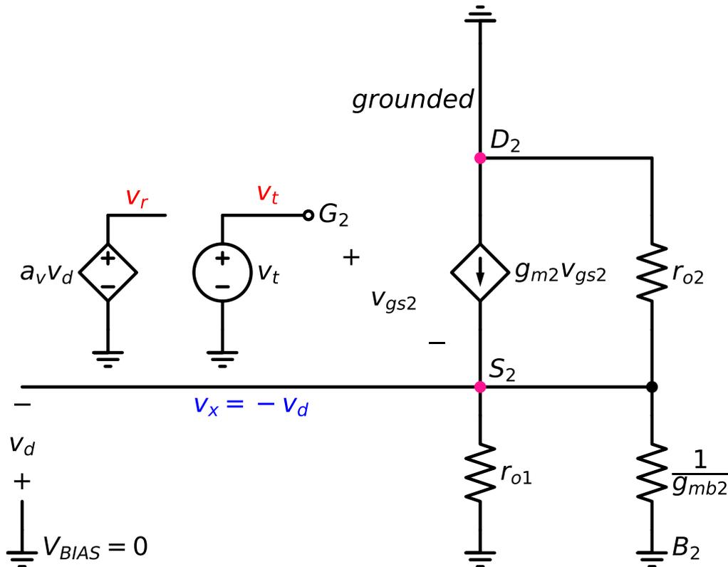
Figure 7.68.: Return ratio for  $a_v$  with the output port shorted
