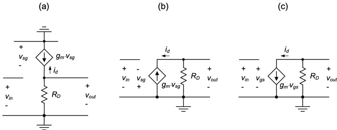
Figure 2.16.: Small-signal model of the p-channel common-source amplifier: (a) using the p-channel model directly, (b) a flipped version of (a), and (c) with sign changes applied to show equivalence with the n-channel model.
