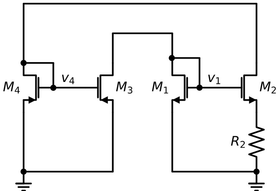
Figure 7.43.: Unrolled AC equivalent model for the constant- $g_m$  bias circuit
