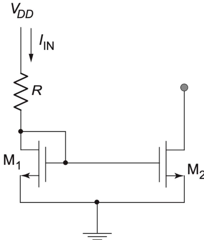
Figure 5.25.: Simple supply-referenced current generator.
