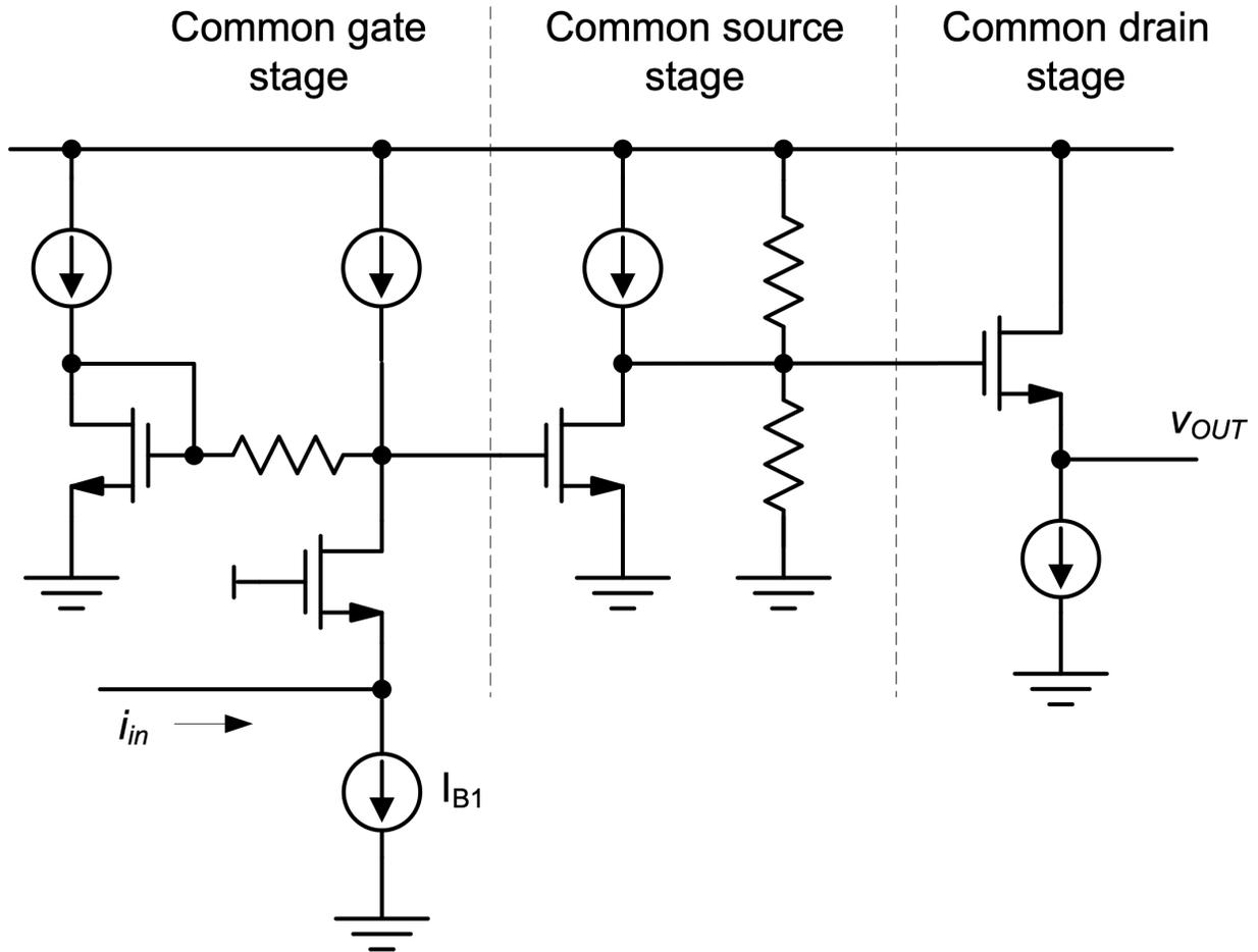
Figure 1.5.: Example realization of a transimpedance amplifier.
