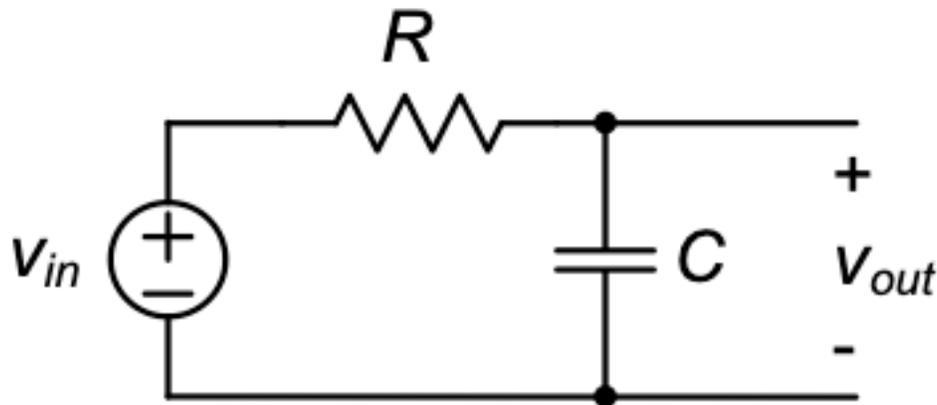
Figure 3.1.: RC circuit example.
