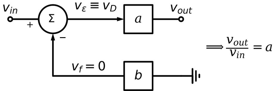
Figure 7.21.: Breaking the loop ( $v_f = 0$ )
