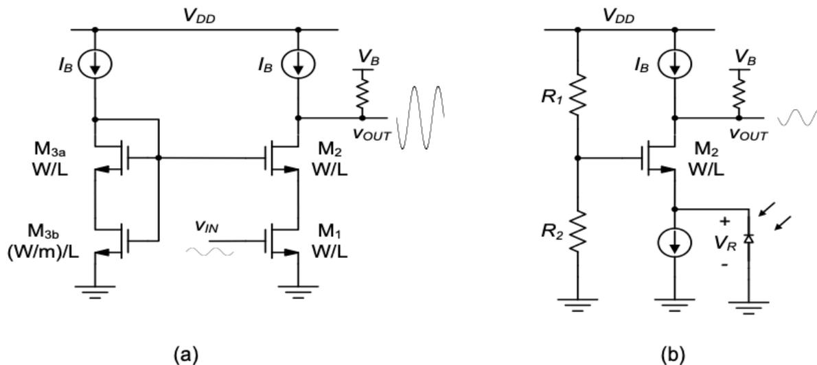
Figure 5.31.: Voltage biasing in two usage cases of a common-gate stage.
