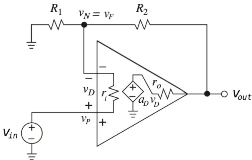
Figure 7.7.: Non inverting voltage amplifier with non ideal op amp (Franco 2015)
