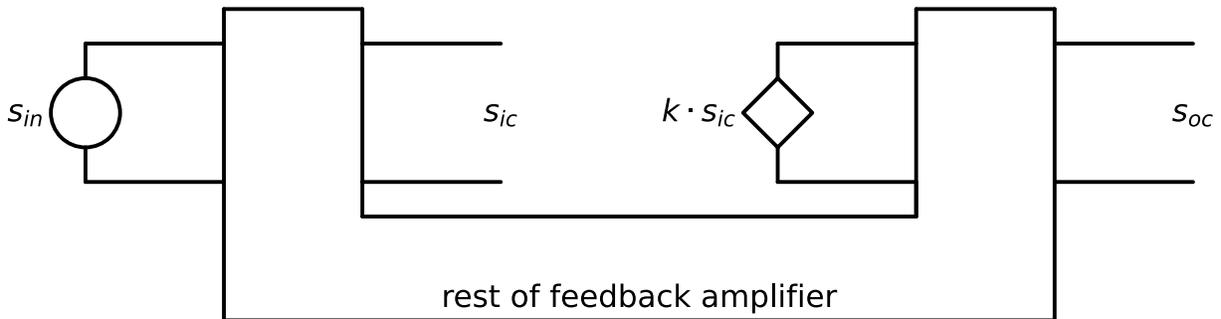
Figure 7.33.: Feedback amplifier: return ratio framework to derive the closed-loop gain
