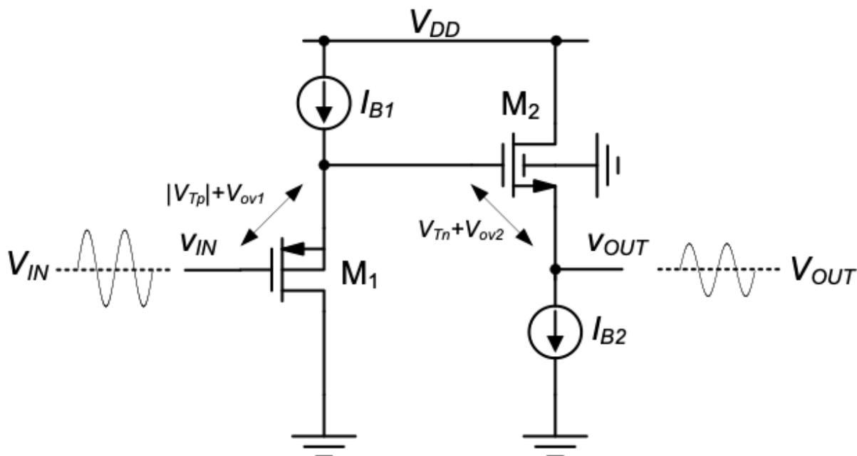
Figure 5.33.: Back-to-back common-drain stages to realize equal input and output quiescent point voltages.
