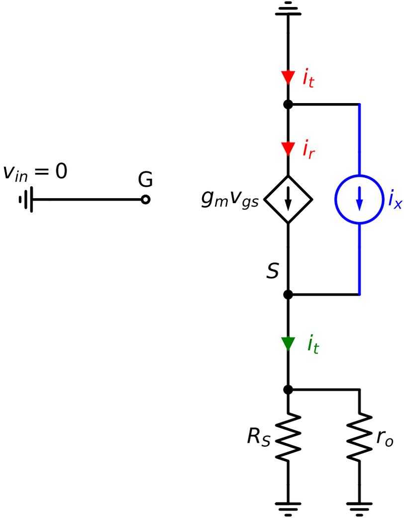
Figure 7.76.: return ratio with output port shorted
