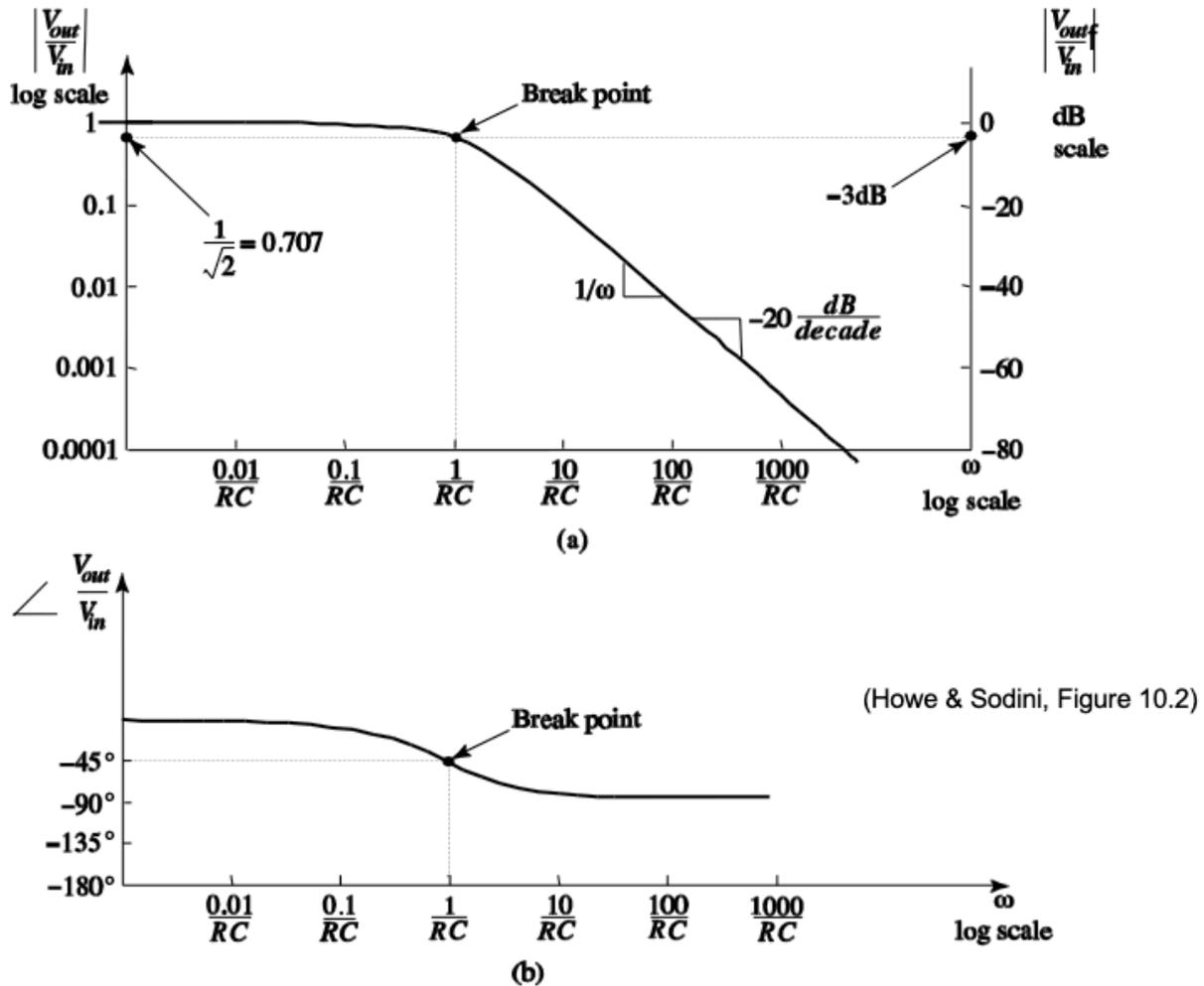
Figure 3.2.: Bode plot for the RC circuit example of Figure 3.1. (a) Log magnitude vs. log frequency. (b) Phase vs. log frequency.
