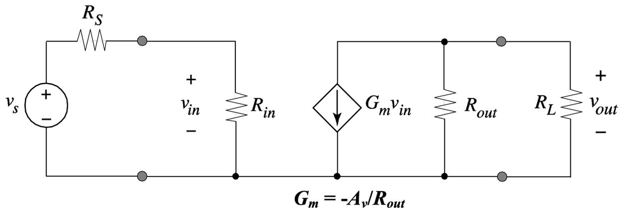
Figure 1.12.: Voltage amplifier with an underlying transconductance amplifier model
