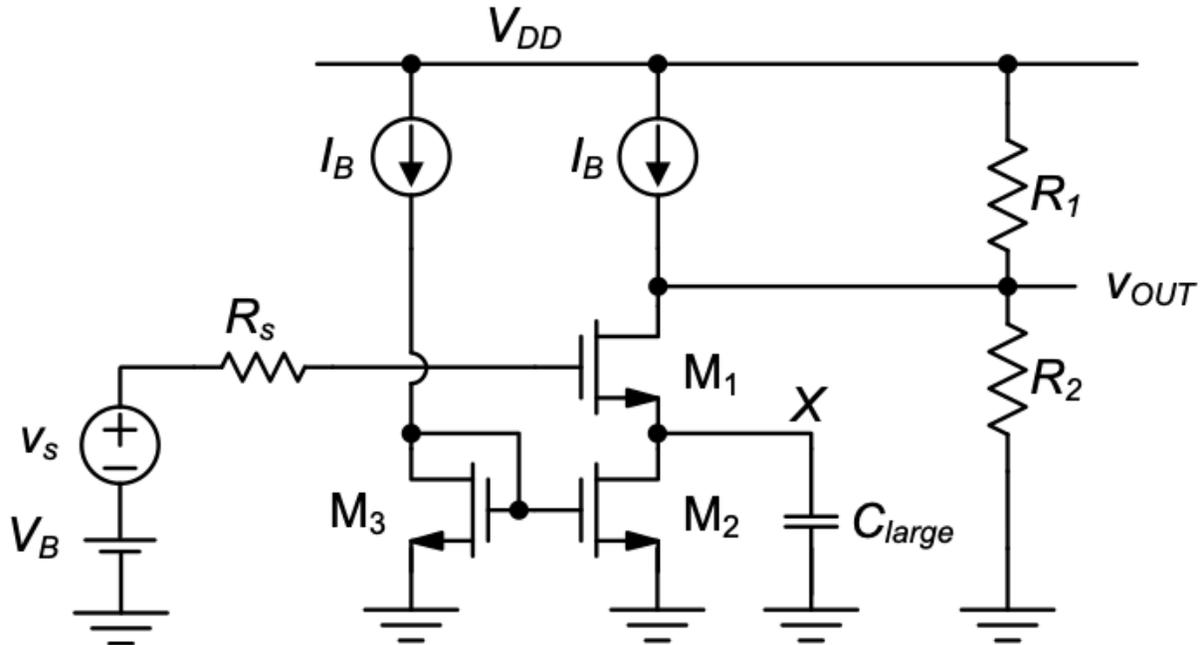
Figure 5.30.: Biasing-approach using AC coupling at the source of a common-source stage.
