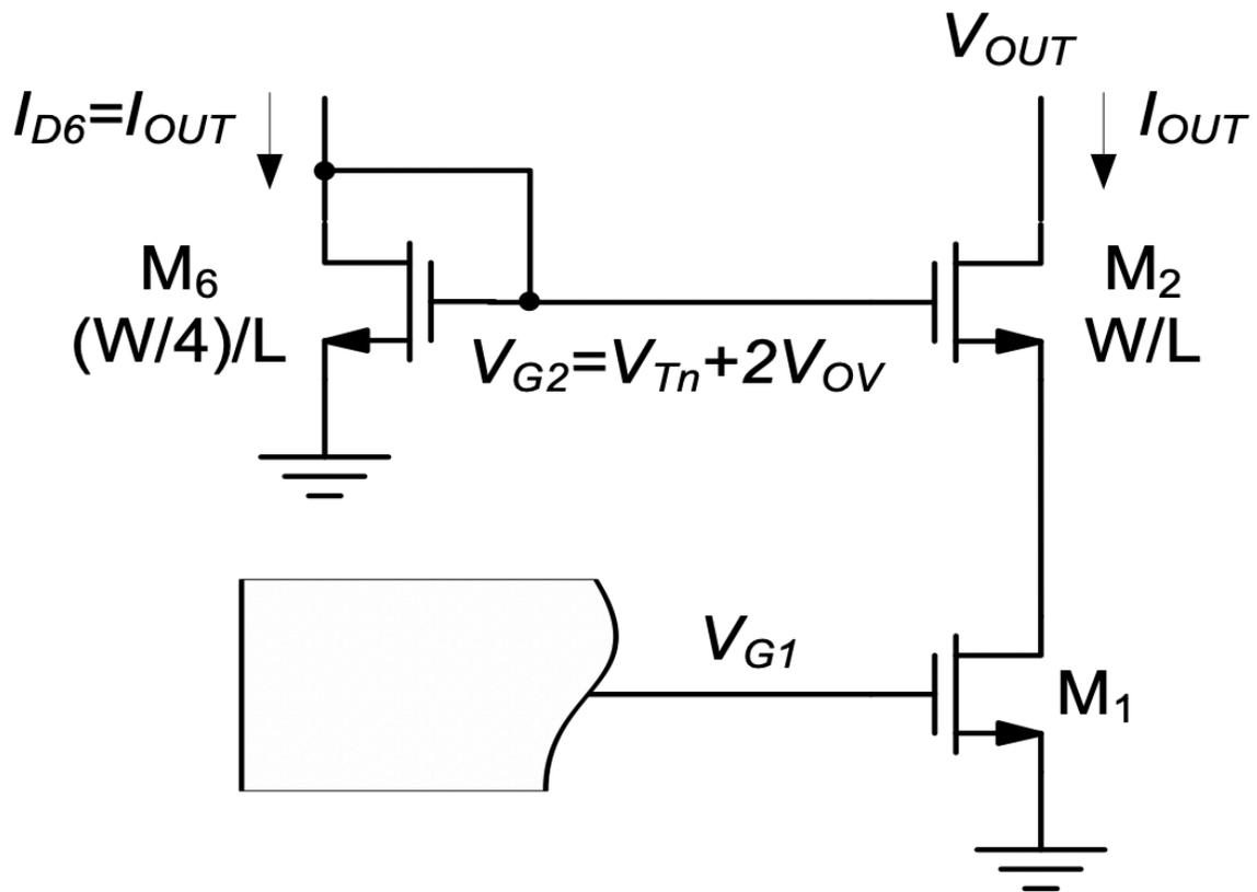
Figure 5.20.: Basic circuit for cascode voltage generation.
