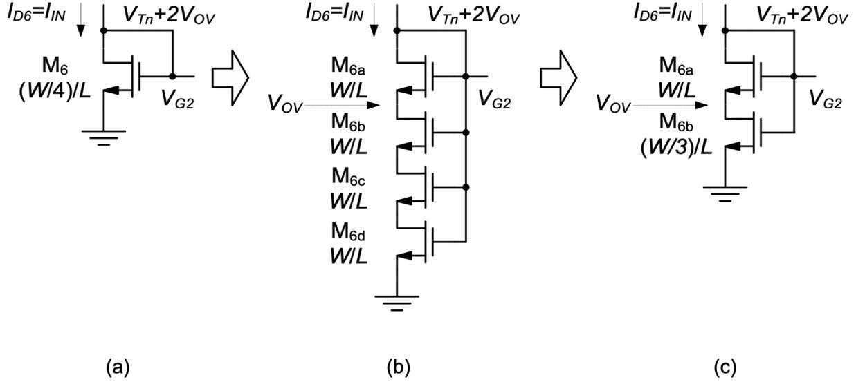
Figure 5.22.: Conceptual steps for replacing the  $W/4$  cascode biasing device with a two-transistor compound circuit
