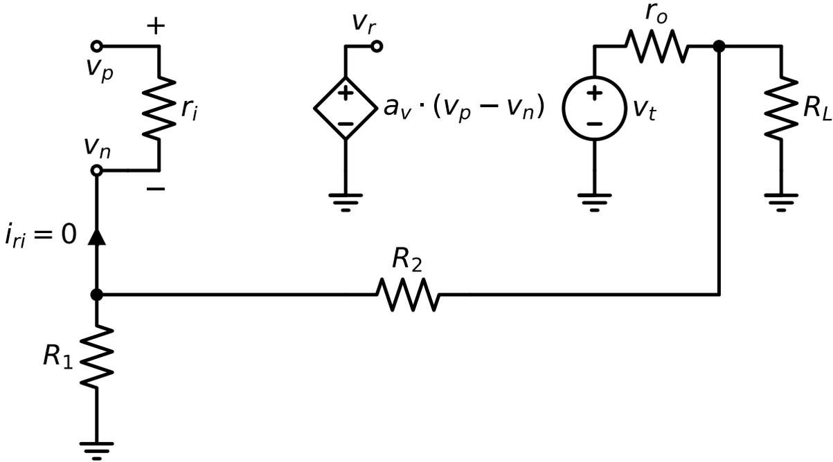
Figure 7.52.:  $T$ (with input port open) for non inverting configuration
