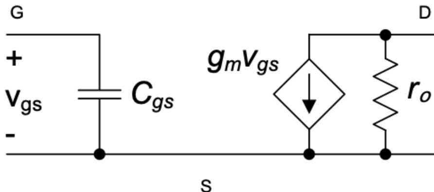
Figure 3.8.: MOSFET small-signal model for the saturation region, including the intrinsic gate capacitance.
