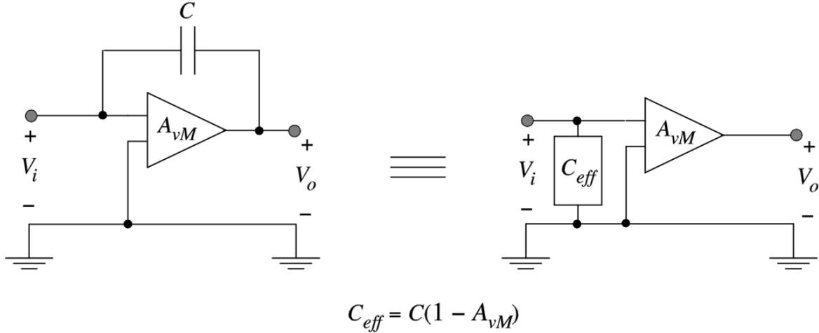
Figure 3.18.: Idealized voltage amplifier with coupling capacitance between its input and output.
