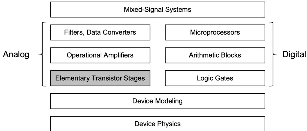
Figure 1.6.: Levels of abstraction in integrated circuit design.
