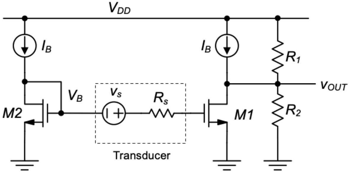
Figure 5.28.: Replica biasing approach for setting up the quiescent point gate-source voltage of a common-source stage.
