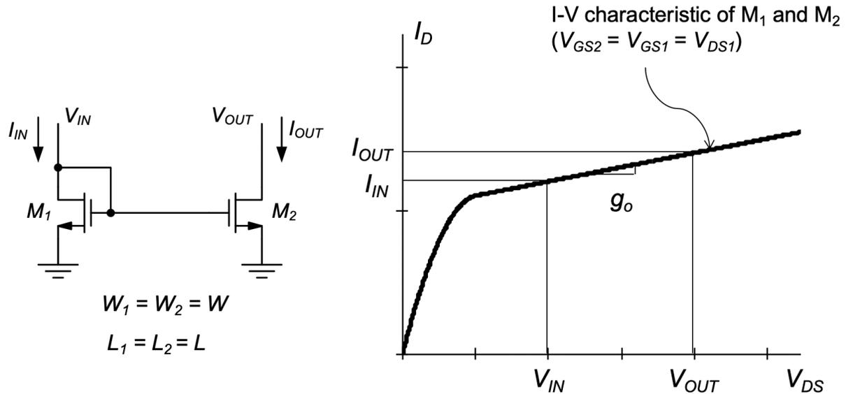
Figure 5.8.: Mirror error due to differences in drain-source voltage.
