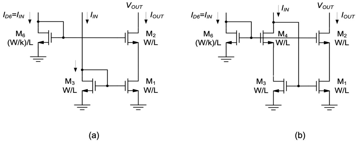
Figure 5.21.: High-swing cascode current mirror with input branch included. (a) Non-preferred solution that suffers from a systematic mirror ratio error. (b) Solution that avoids the systematic mirror ratio error.
