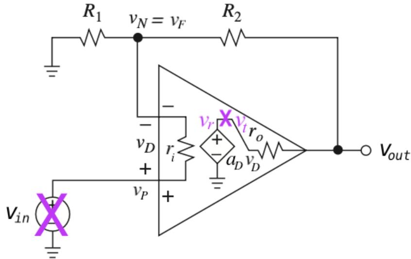
Figure 7.18.: Non inverting op amp amplifier with  $v_{in}$  nulled and the loop broken at the opamp's vcvs.
