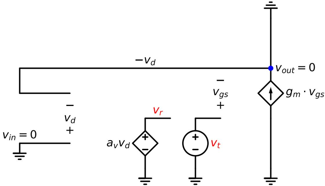
Figure 7.57.: Finding T (with output port shorted),  $-v_d = v_{out} = 0$
