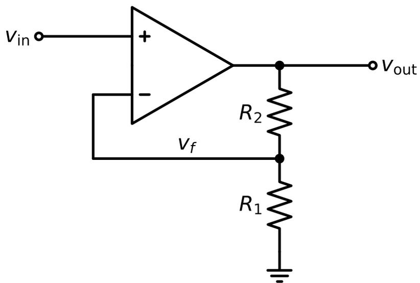
Figure 7.6.: op amp based non inverting voltage amplifier
