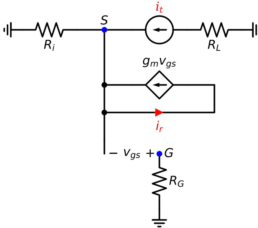
Figure 7.71.: return ratio with port G-S open
