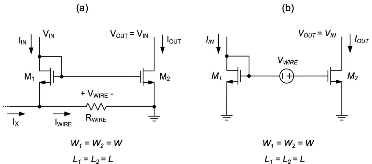
Figure 5.9.: Mirror error due to voltage drop in the source connection.
