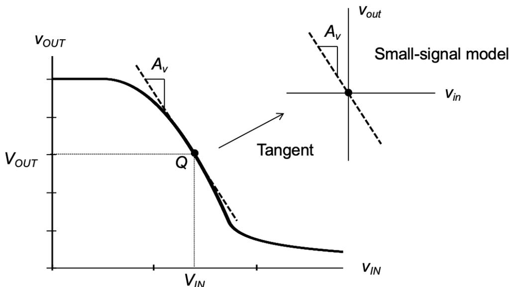
Figure 2.11.: Concept of small-signal voltage gain. In the small signal model, the input and output voltages are linearly related through  $A_v$ , the slope of the tangent at the operating point of the large-signal transfer characteristic.
