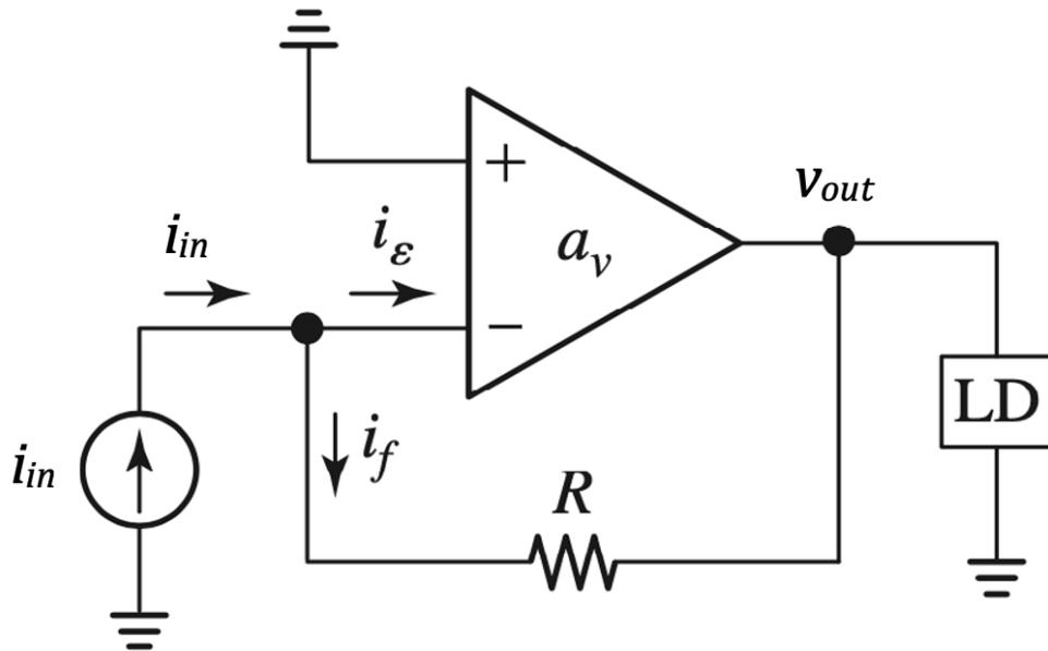
Figure 7.28.: Shunt-shunt configuration:  $b = \frac{i_f}{v_{out}} = -\frac{1}{R}$
