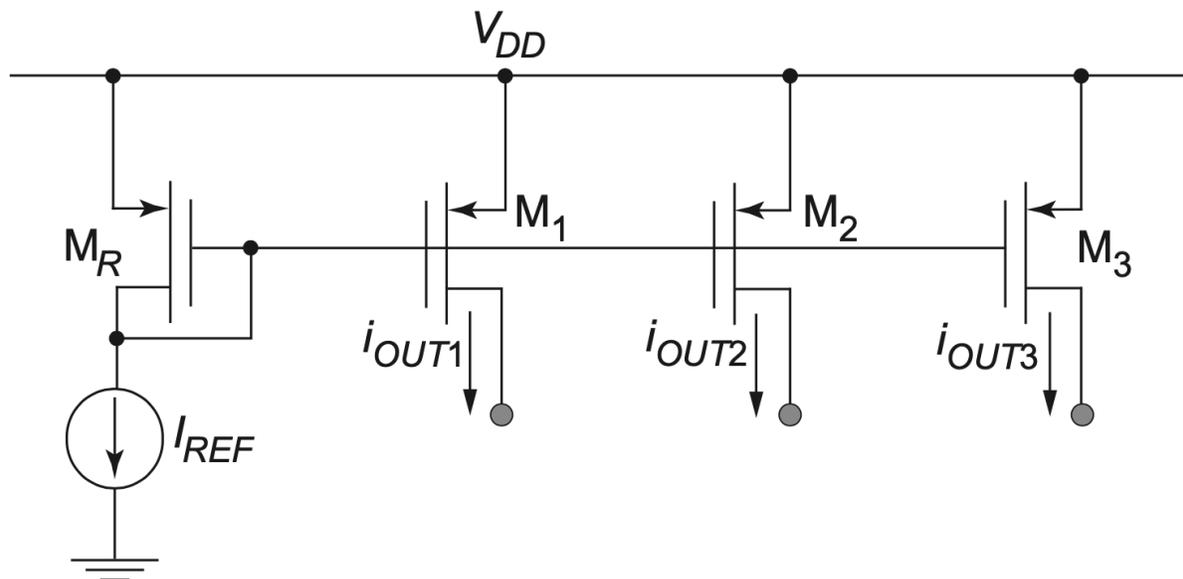
Figure 5.10.: PMOS current mirror with multiple outputs.
