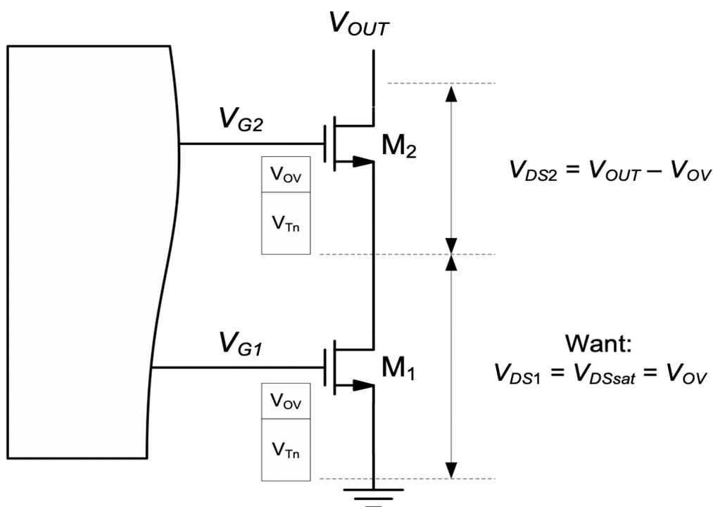
Figure 5.19.: Desired output branch biasing to achieve the minimum possible compliance voltage.
