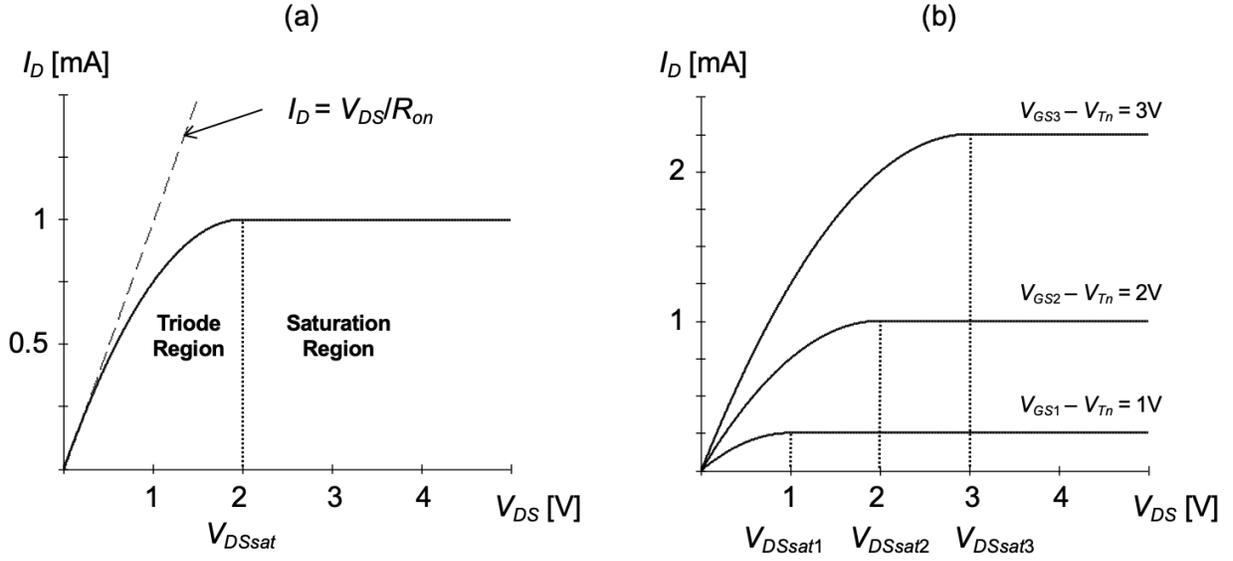
Figure 2.4.: (a) n-channel I-V characteristic for a fixed value of  $V_{GS} - V_{Tn} = 2V$ . (b) I-V plots with varying  $V_{GS} - V_{Tn}$  (drain characteristic). Parameters:  $\mu C_{ox} = 50 \mu A/V^2$  and  $W/L = 10$ .
