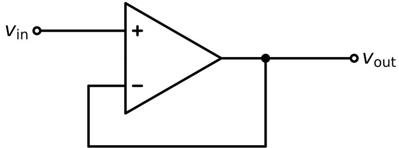
Figure 7.4.: op amp based voltage buffer
