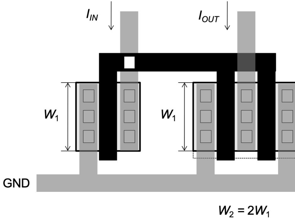
Figure 5.7.: Layout of a current mirror with shared drain regions.
