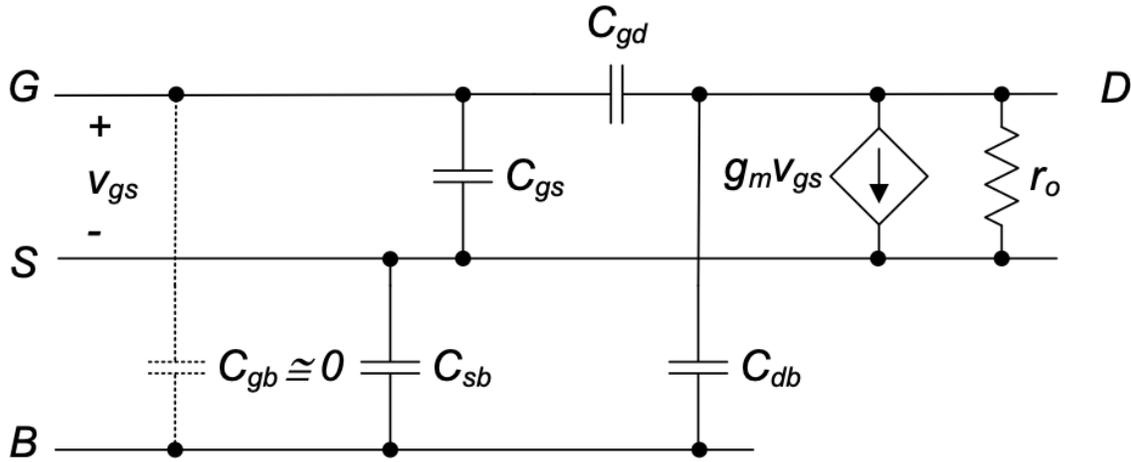
Figure 3.14.: Small-signal model for the n-channel MOSFET in saturation, including intrinsic and extrinsic capacitances.
