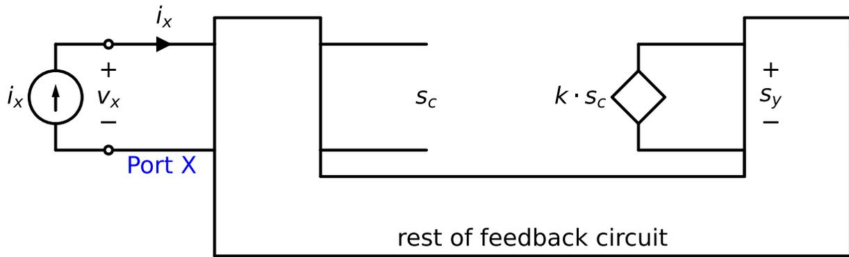
Figure 7.49.: Feedback circuit to derive Blackman's formula with respect to port x
