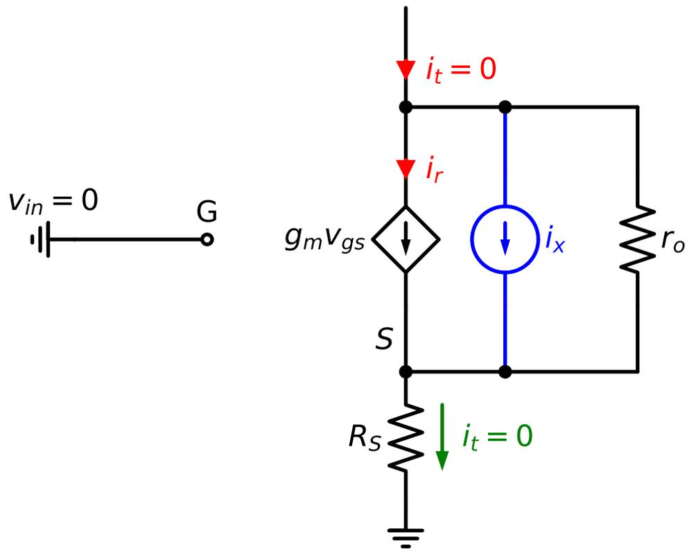
Figure 7.75.: return ratio with output port open
