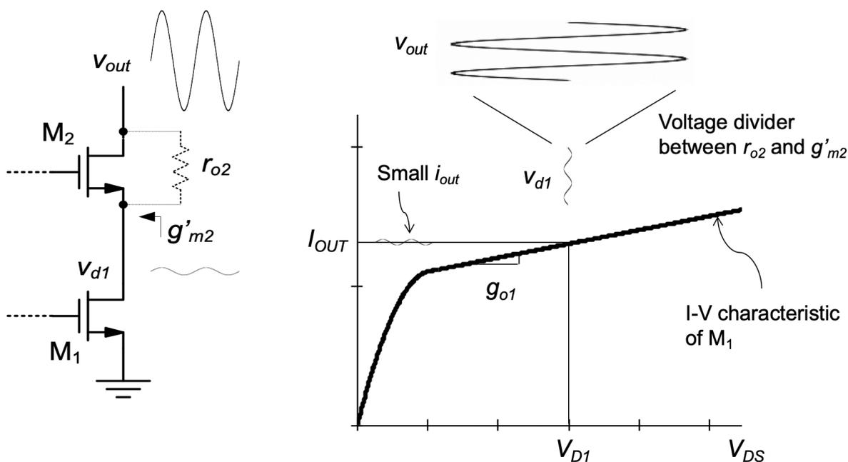
Figure 5.14.: Qualitative inspection of the output branch in a cascode current mirror.
