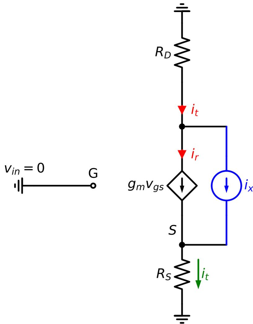
Figure 7.73.: Small signal model to find the return ratio of  $g_m$
