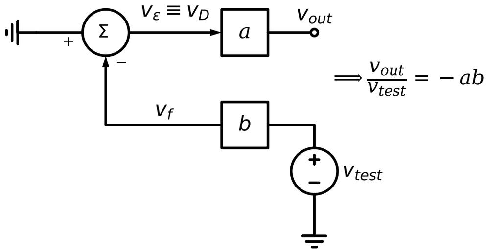
Figure 7.22.: Breaking the loop ( $v_{in} = 0$ )
