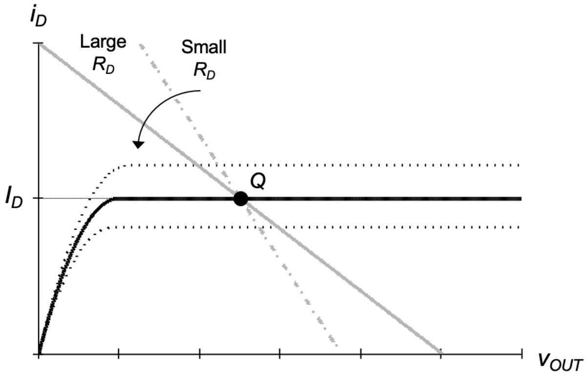
Figure 2.19.: Desired load line behavior.
