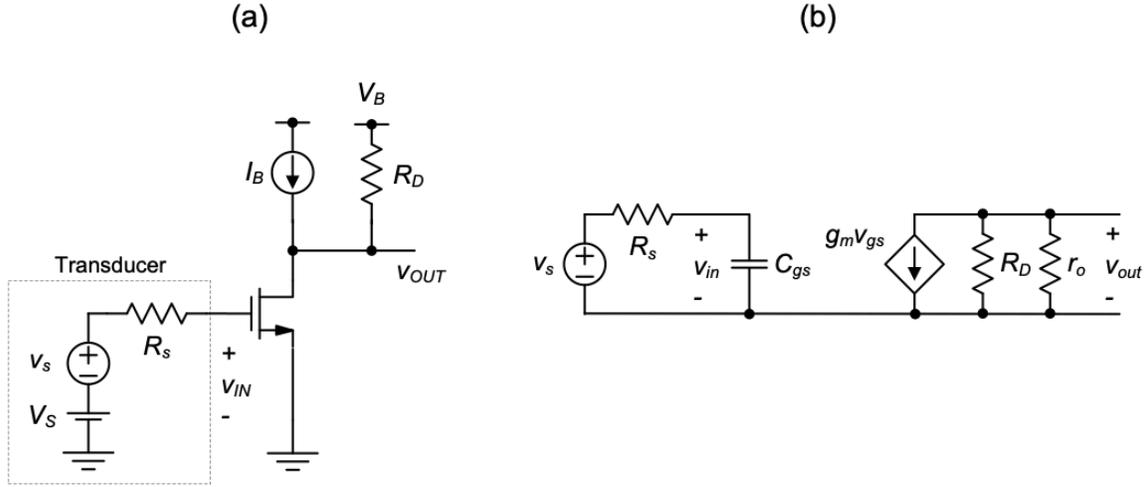
Figure 3.9.: (a) Common-source amplifier driven by a transducer with finite source resistance. (b) Small-signal model with the intrinsic gate capacitance.
