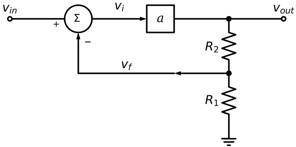
Figure 7.5.: Block diagram of a non inverting voltage amplifier (series-shunt feedback)
