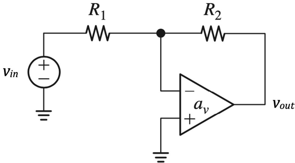
Figure 7.29.: inverting op amp based voltage amplifier
