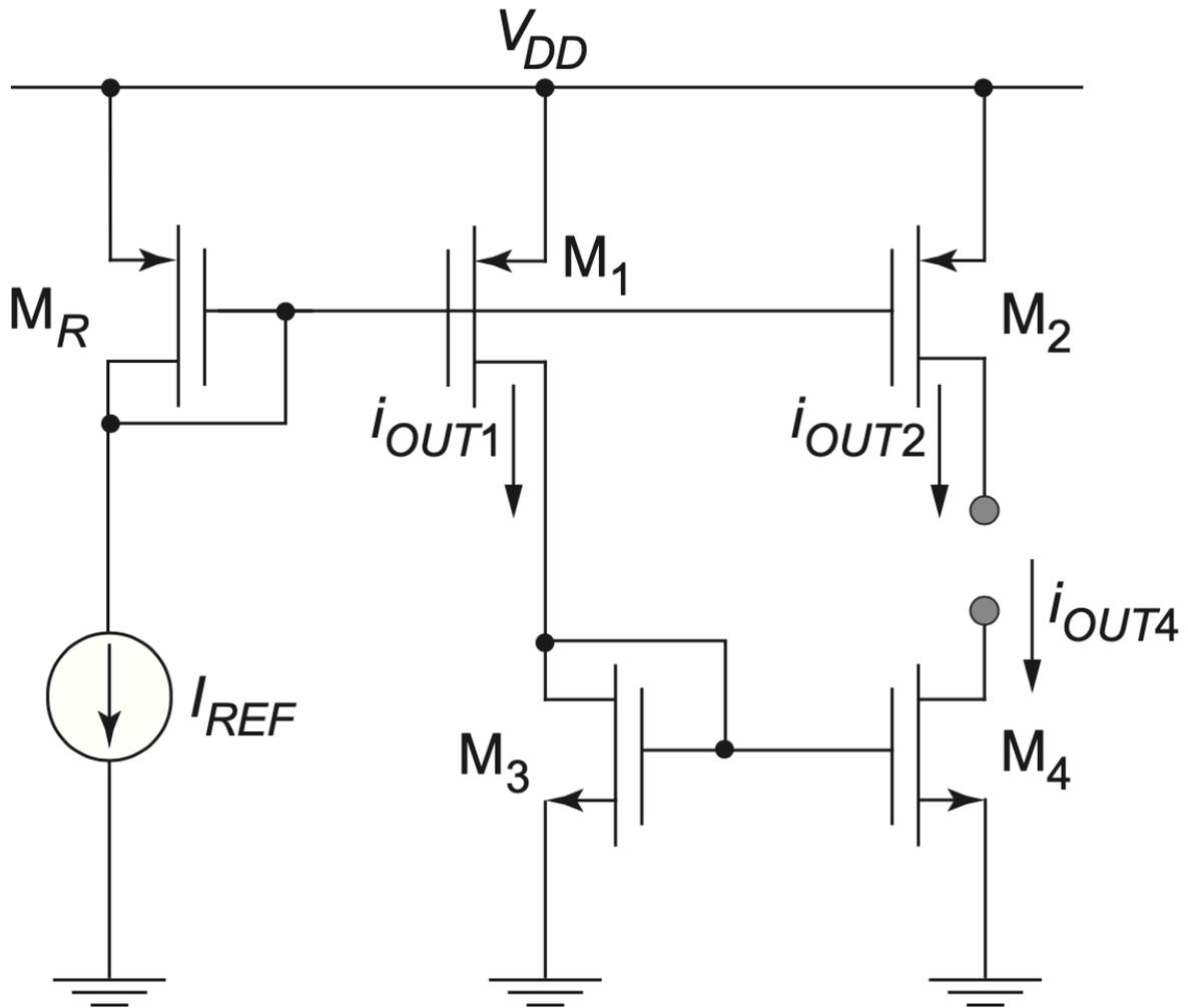
Figure 5.11.: Circuit to produce a current source  $M_2$  and current sink  $M_4$ .
