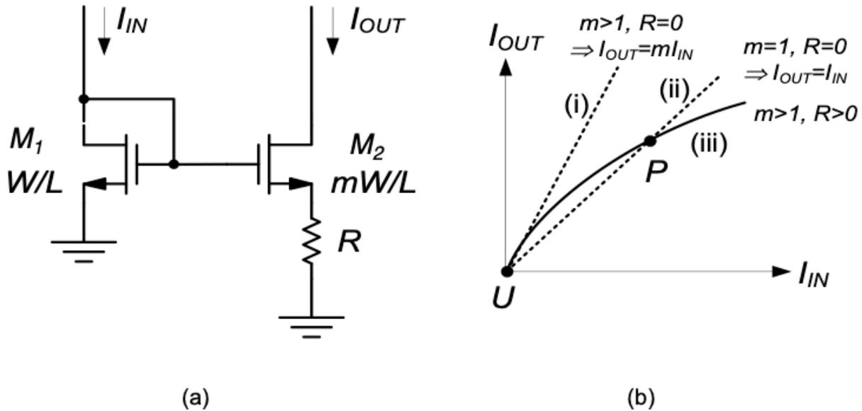
Figure 5.26.: (a) Core building block of a constant-gm current generator. (b) Current transfer characteristics for various scenarios.
