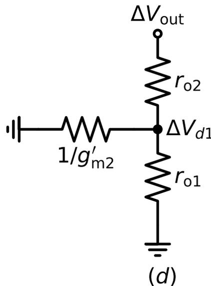
Figure 5.16.: (d) voltage divider between  $r_{o2}$  and  $1/g'_{m2} \parallel r_{o1}$
