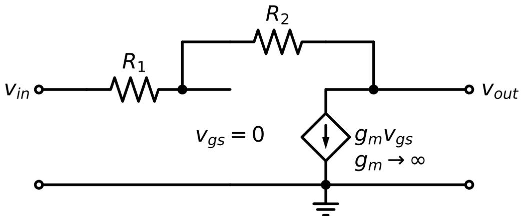
Figure 7.39.: Ideal closed loop gain calculation
