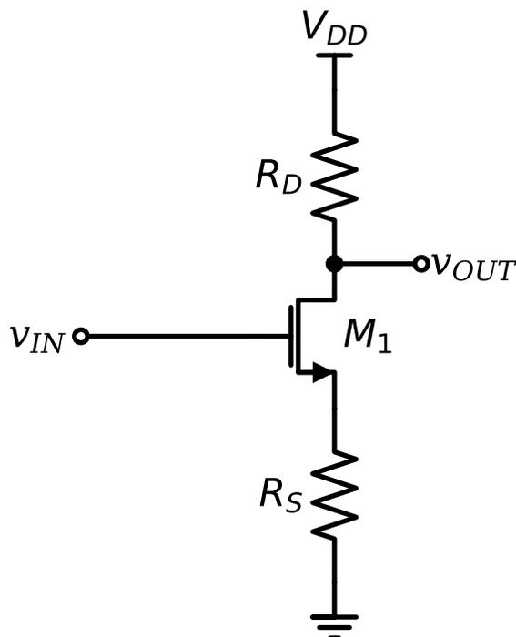
Figure 7.72.: Common source with degeneration
