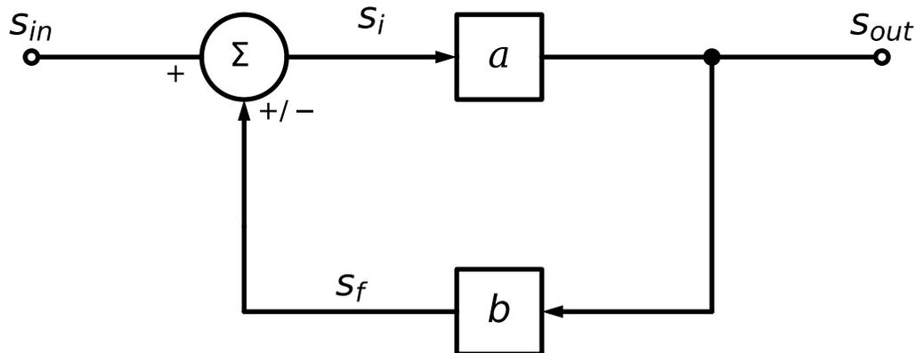
Figure 7.1.: Block diagram of a feedback system.
