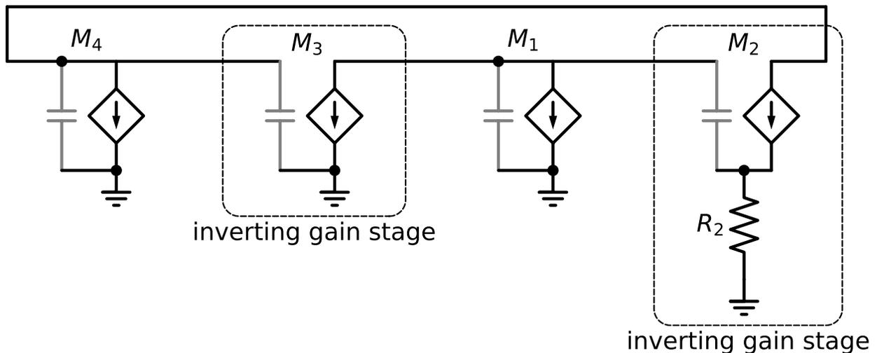
Figure 7.46.: Small signal equivalent model for the constant- $g_m$  bias circuit
