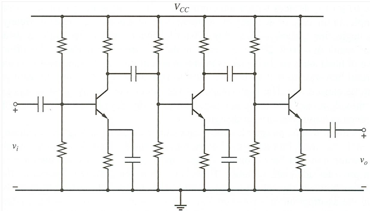
Figure 1.18.: Example of a discrete amplifier circuit using bipolar junction transistors (BJTs).
