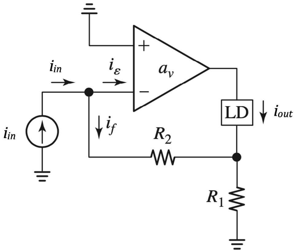
Figure 7.32.: shunt-series configuration:  $b = \frac{i_f}{i_{out}} = -\frac{R_1}{R_1 + R_2} = -\frac{1}{1 + R_2/R_1}$
