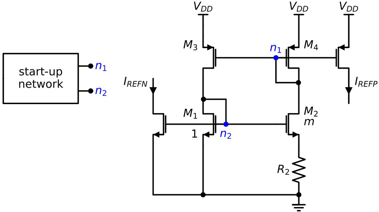
Figure 7.47.: Constant- $g_m$  reference: design example
