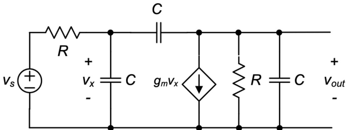
Figure 3.25.: Circuit example with three open-circuit time constants.
