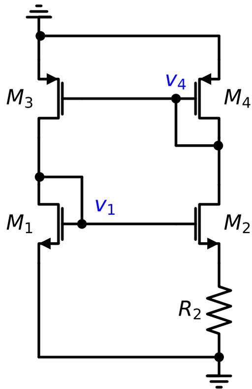
Figure 7.42.: AC equivalent model of the constant- $g_m$  bias circuit
