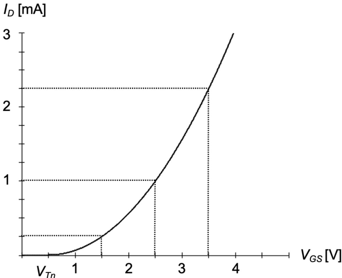
Figure 2.5.: Plot of n-channel drain current as a function of  $V_{GS}$  (transfer characteristic). Parameters:  $V_{DS} = 5$  V,  $\mu C_{ox} = 50$  A/V<sup>2</sup>,  $V_{Tn} = 0.5$  V, and  $W/L = 10$ .
