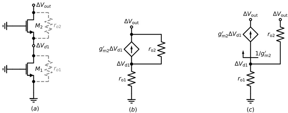
Figure 5.15.: (a) cascode with voltage perturbation applied at its output (b) & (c) equivalent small signal model
