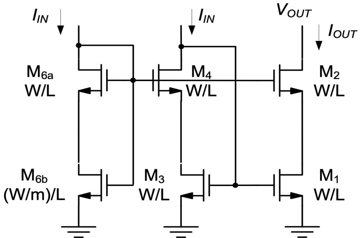
Figure 5.23.: Complete high-swing cascode current mirror using a triode device ( $M_{6b}$ ) for cascode biasing.
