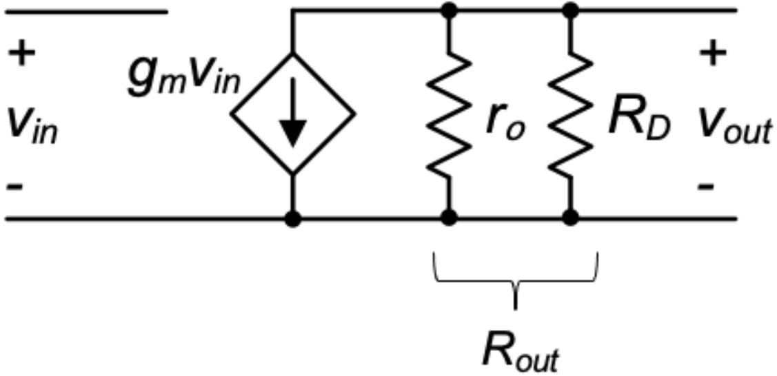
Figure 2.25.: Small-signal model for the circuit of Figure 2.20(a), with finite output conductance.
