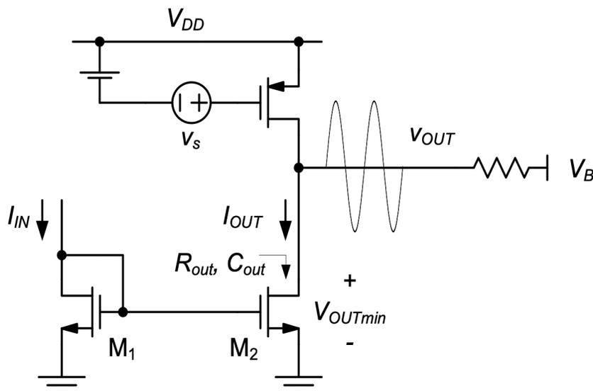
Figure 5.4.: Application of the basic current mirror in a common-source amplifier.
