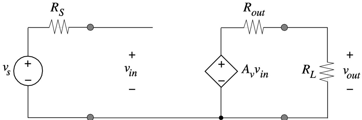
Figure 2.27.: Common-source amplifier model with transducer and load resistance.
