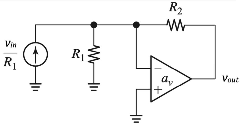
Figure 7.30.: inverting op amp based voltage amplifier with the input voltage source transformed into a current source
