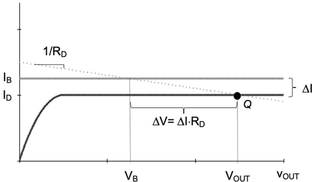
Figure 2.21.: Bias point shift due to mismatch in  $I_B$  and  $I_D$ .
