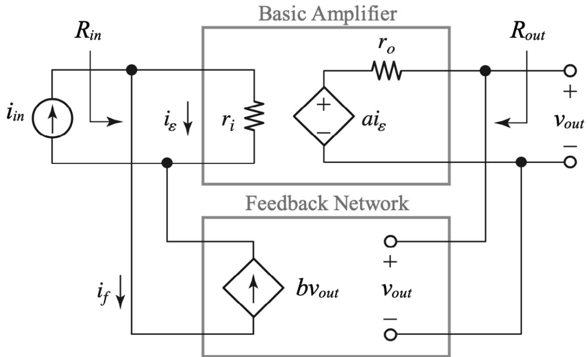
Figure 7.12.: The ideal shunt-shunt configuration or transimpedance amplifier (Franco 2015)
