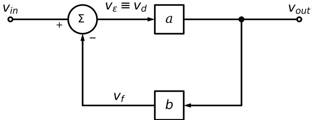
Figure 7.15.: Block diagram of negative feedback system.
