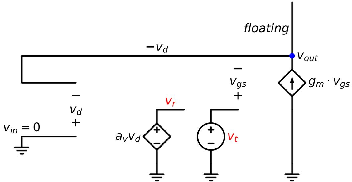
Figure 7.58.: Finding T (with output port open),  $v_{out} = -v_d = -v_{gs} + v_t$
