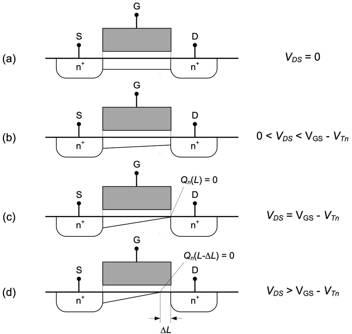
Figure 2.3.: Channel profile for varying  $V_{DS}$ .
