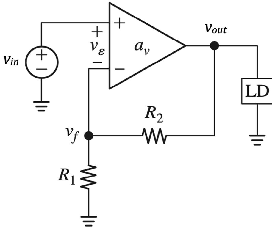
Figure 7.27.: Series-shunt configuration:  $b = \frac{v_f}{v_{out}} = \frac{R_1}{R_1 + R_2}$
