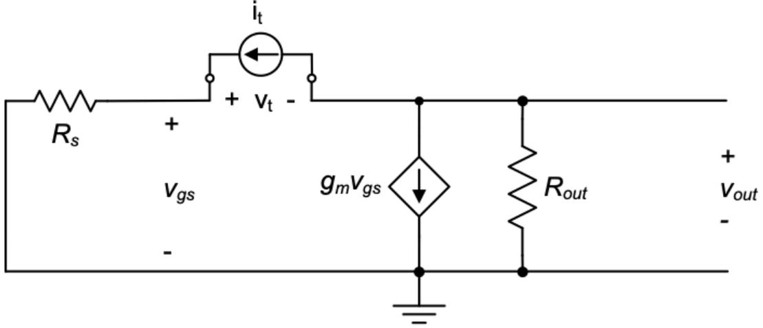
Figure 3.22.: Circuit to determine the Thévenin resistance seen across  $C_{gd}$ .
