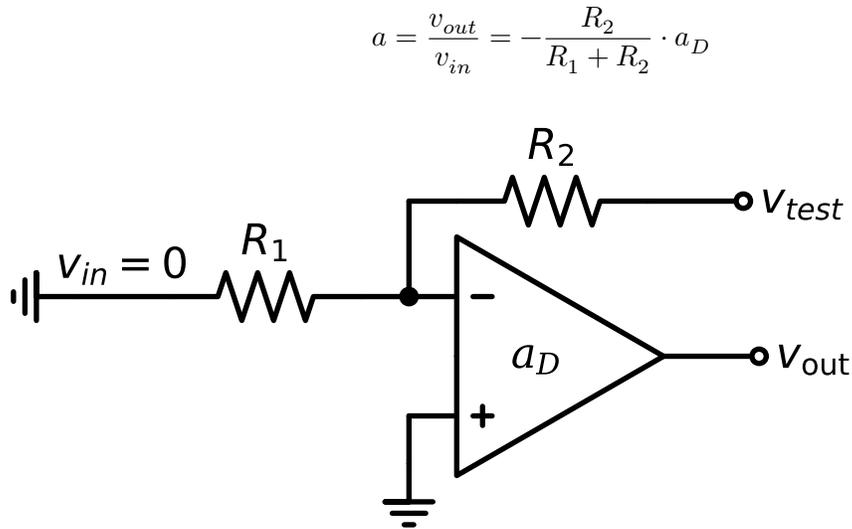
Figure 7.24.: op amp based inverting amplifier with break in the loop ( $v_{in} = 0$ )
