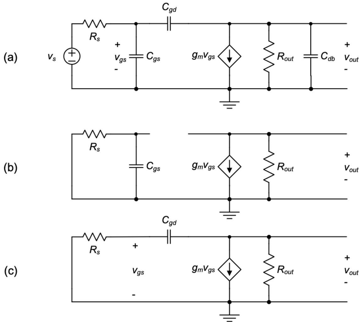
Figure 3.21.: OCT analysis for a common-source amplifier. (a) Complete circuit. (b) Circuit for finding  $\tau_{g_s}$ . (c) Circuit for finding  $\tau_{g_d}$ .
