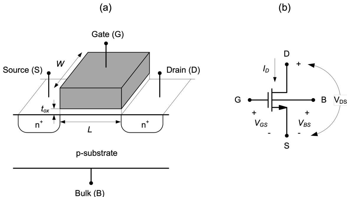
Figure 2.1.: (a) Cross-section of an n-channel MOSFET.
