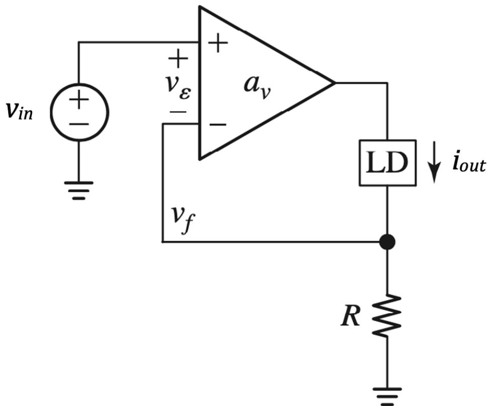
Figure 7.31.: series-series configuration:  $b = \frac{v_f}{i_{out}} = R$
