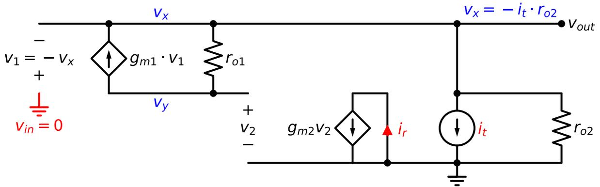
Figure 7.62.: Return Ratio for  $g_{m2}$  with the output port open
