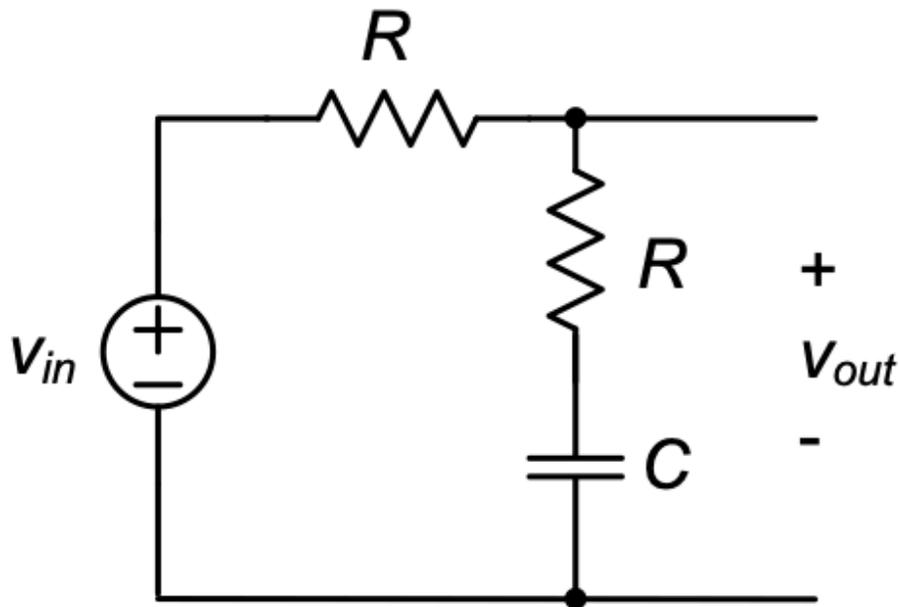
Figure 3.3.: RC circuit with series resistor.
