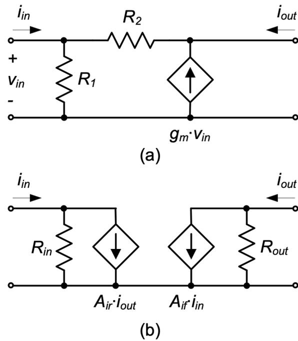
Figure 1.13.: (a) Example of a bilateral current amplifier. (b) Corresponding bilateral current amplifier two-port model.
