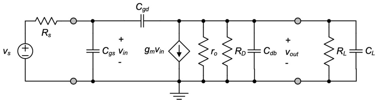
Figure 3.26.: General two-port model for the common-source voltage amplifier valid at high frequencies.
