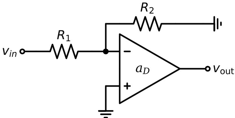
Figure 7.23.: op amp based inverting amplifier with break in the loop ( $v_f = 0$ )
