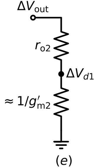
Figure 5.17.: (e) voltage divider between  $r_{o2}$  and  $1/g'_{m2}$
