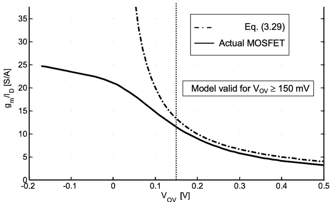
Figure 2.17.: Transconductance to current ratio predicted by Equation 2.31 and the behavior of an actual MOSFET.
