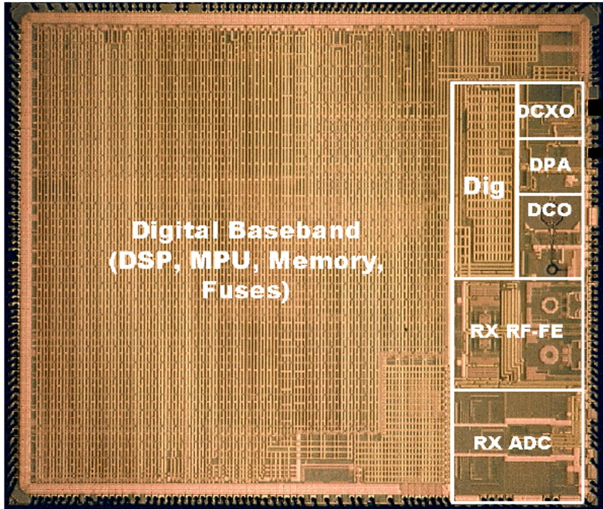
Figure 1.3.: Chip photo of a single-chip radio (Staszewski et al. 2008).
