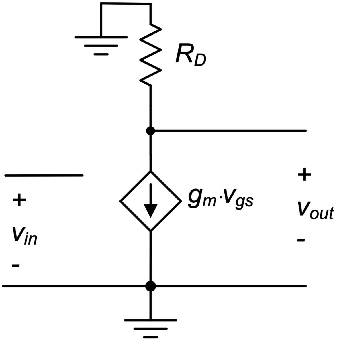
Figure 2.14.: Small-signal model of the circuit in Figure 2.7(a).
