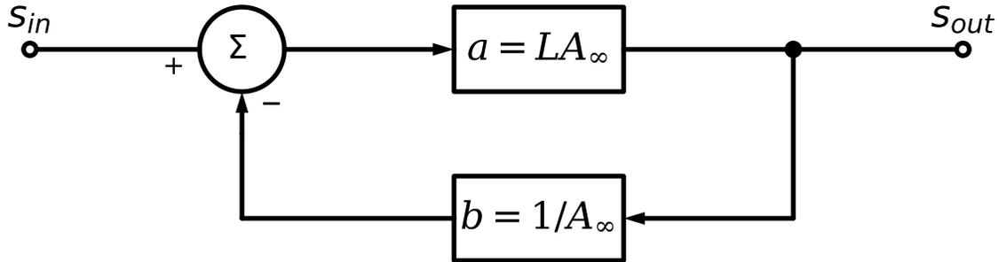
Figure 7.35.: Block diagram model for closed-loop gain using the two-port framework
