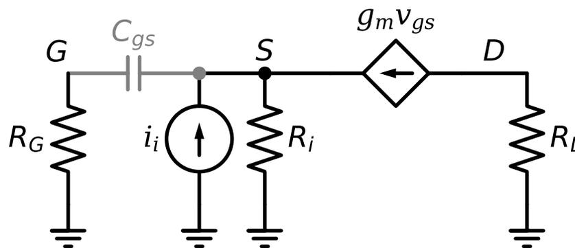
Figure 7.70.: Small signal model for ZVTC calculations, assuming  $r_o$  can be ignored
