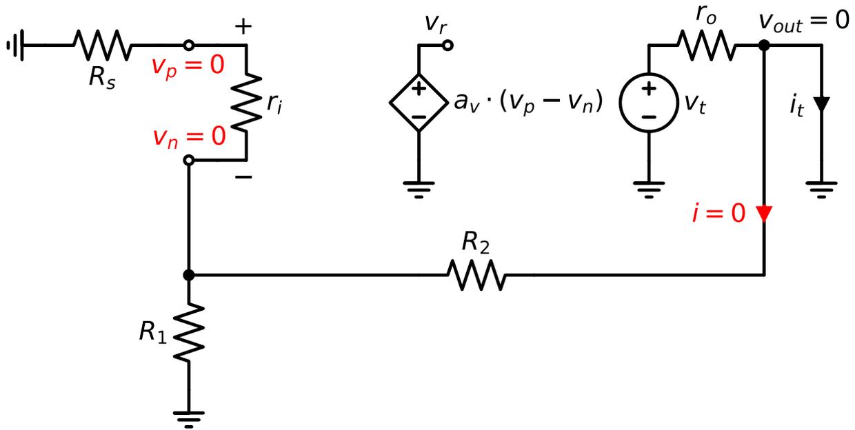
Figure 7.54.:  $T$  (with output port shorted) for non-inverting configuration
