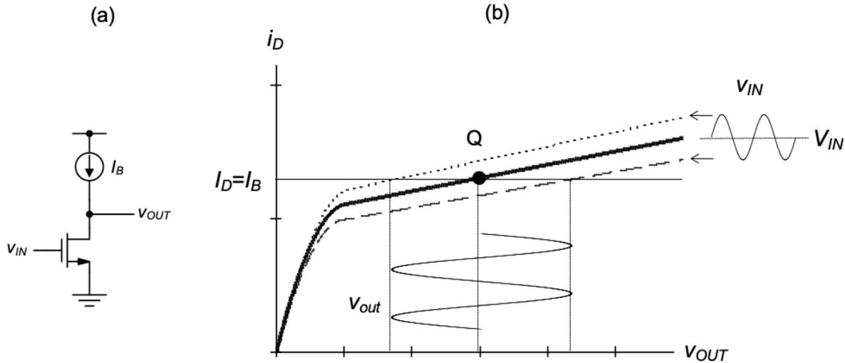
Figure 2.23.: (a) Intrinsic voltage gain stage. (b) Load line plot.
