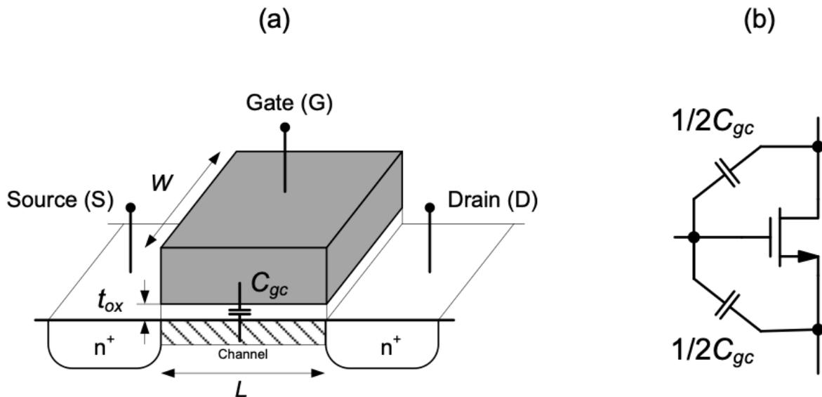
Figure 3.7.: (a) MOSFET cross-section showing the intrinsic capacitance between the gate and the channel ( $C_{gc}$ ). (b) Capacitance model for the triode region.
