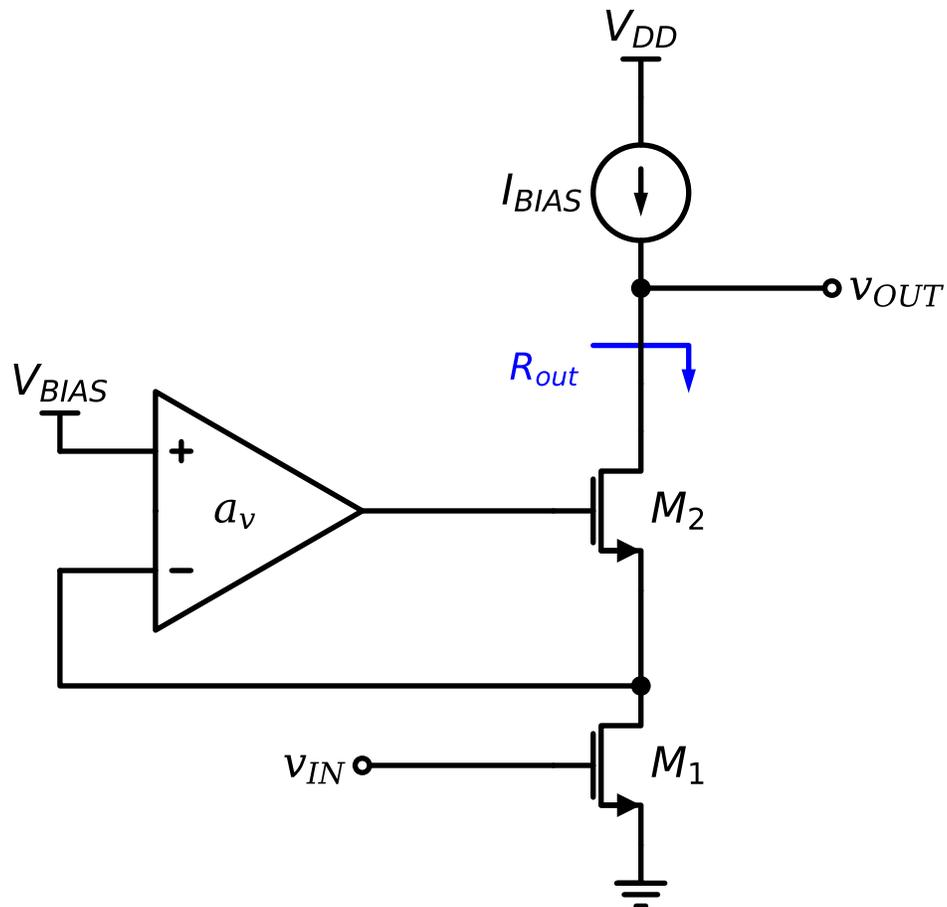
Figure 7.66.: Active cascode gain stage
