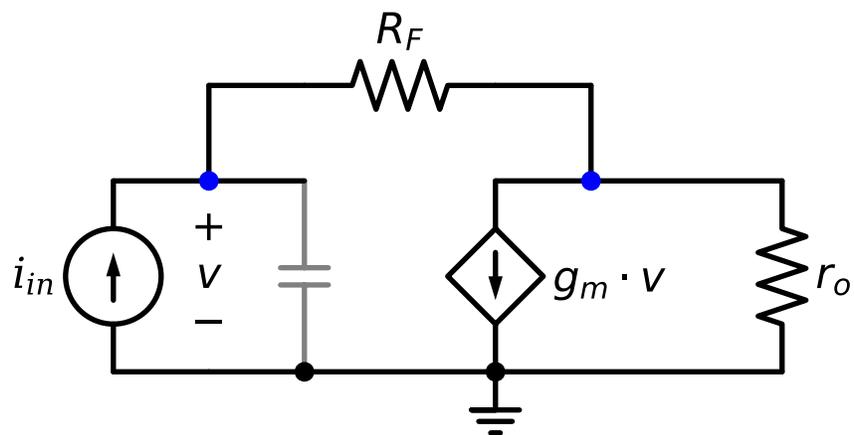
Figure 7.64.: Small signal model of the shunt-shunt stage
