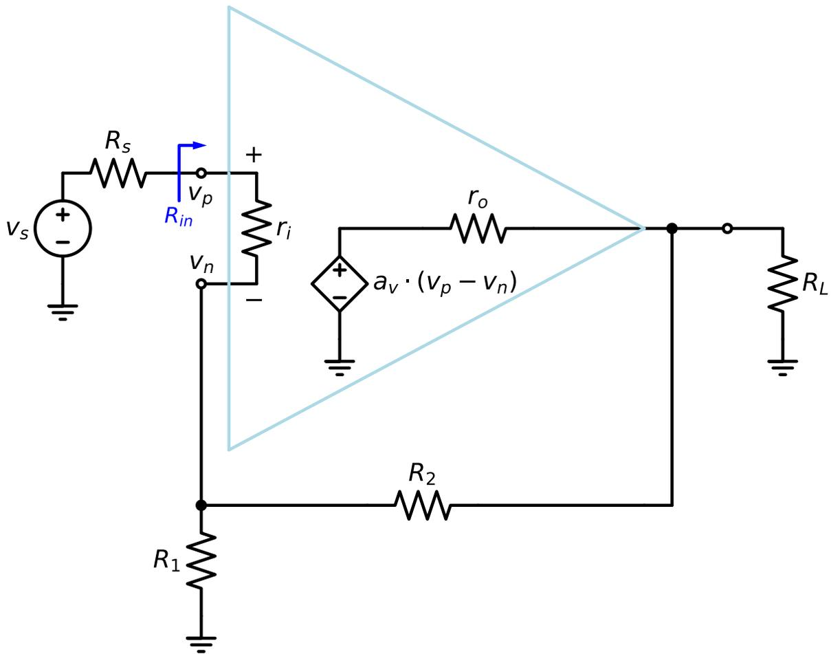
Figure 7.50.: Input resistance of non-inverting op amp circuit
