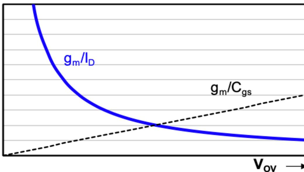
Figure 3.10.: Tradeoff between  $g_m/I_D$  and  $g_m/C_{gs}$ .
