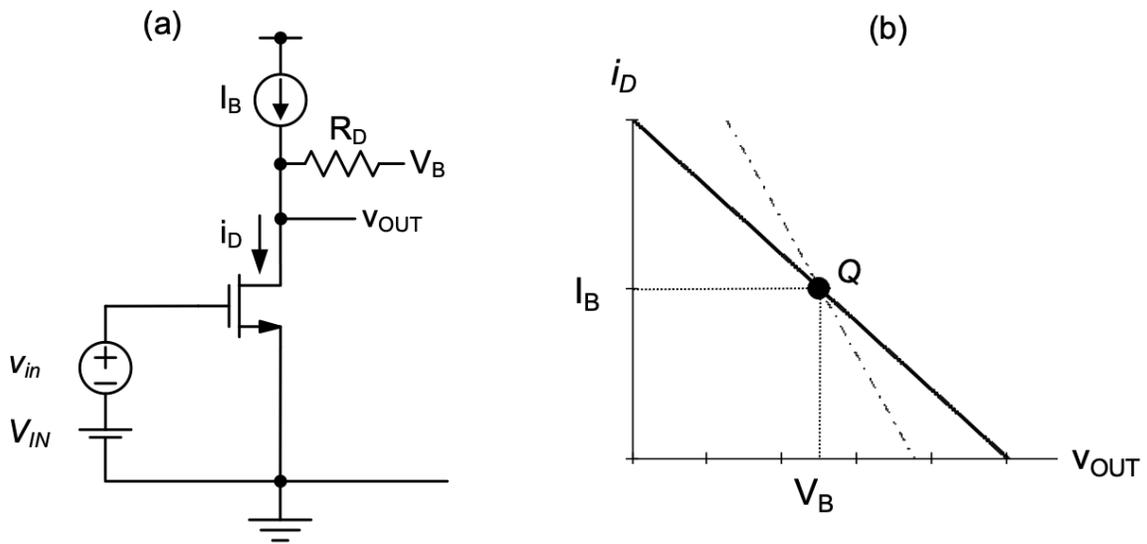
Figure 2.20.: (a) CS amplifier with modified drain biasing scheme. (b) Load line characteristic.
