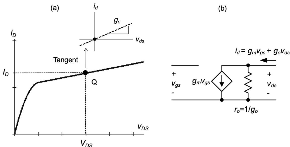
Figure 2.24.: (a) Graphical interpretation of  $g_o$ . (b) MOSFET small-signal model for the saturation region with output conductance ( $g_o$ ).
