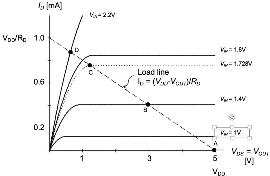
Figure 2.8.: Load line plot for the CS amplifier in Figure 2.7(a). Parameters:  $V_{DD} = 5 \text{ V}$ ,  $R_D = 5 \text{ k}\Omega$ , and  $W/L = 20$ .
