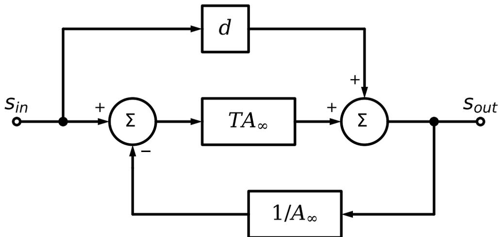
Figure 7.34.: Block diagram for closed-loop gain using return ratio framework
