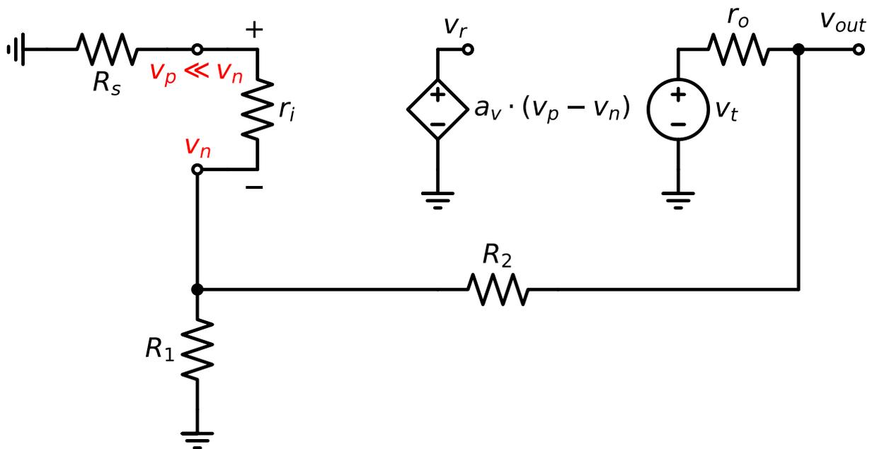
Figure 7.55.:  $T$  (with output port open) for non-inverting configuration
