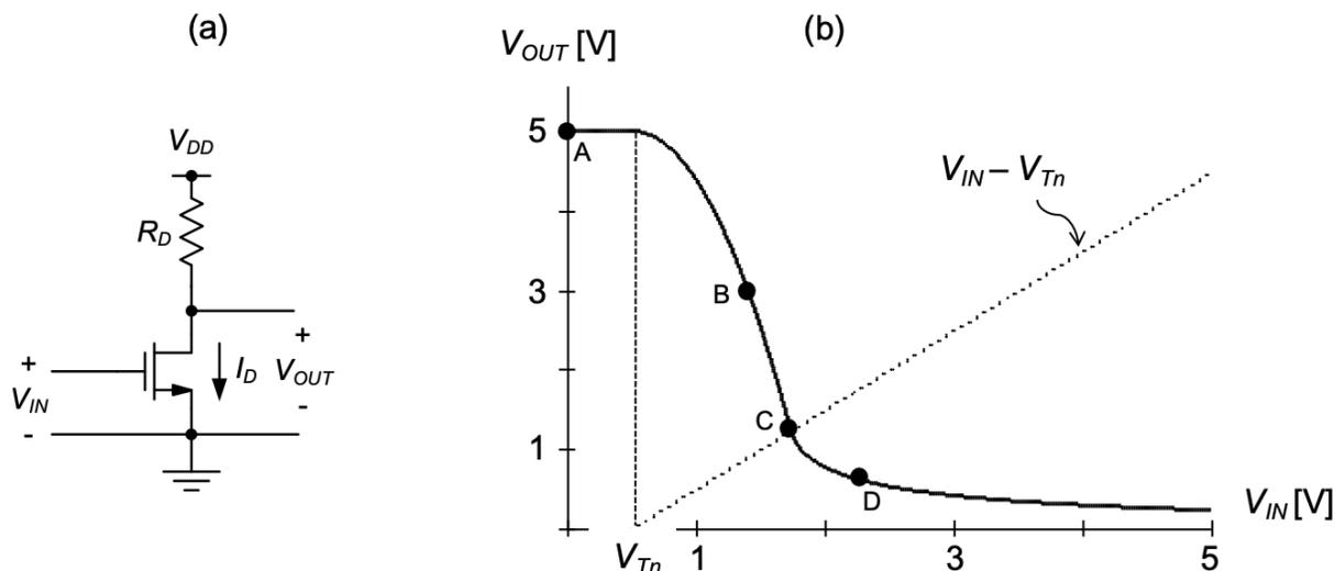
Figure 2.7.: (a) Basic common-source amplifier schematic. (b) Voltage transfer characteristic for  $V_{DD} = 5$  V,  $R_D = 5$  k $\Omega$ , and  $W/L = 20$ .
