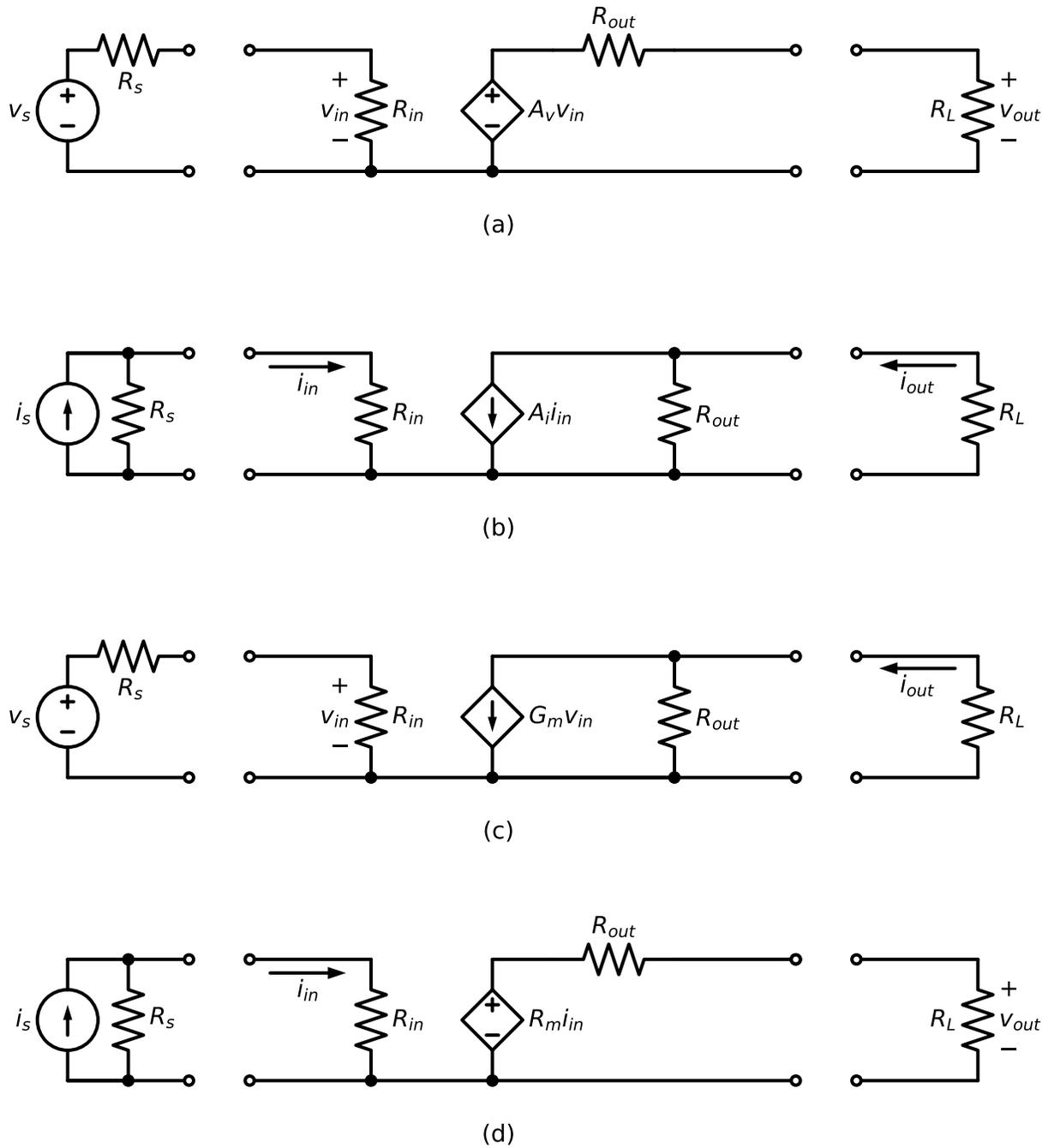
Figure 1.9.: Two-port amplifier models with input source and load: (a) voltage amplifier, (b) current amplifier, (c) transconductance amplifier, and (d) transresistance amplifier
