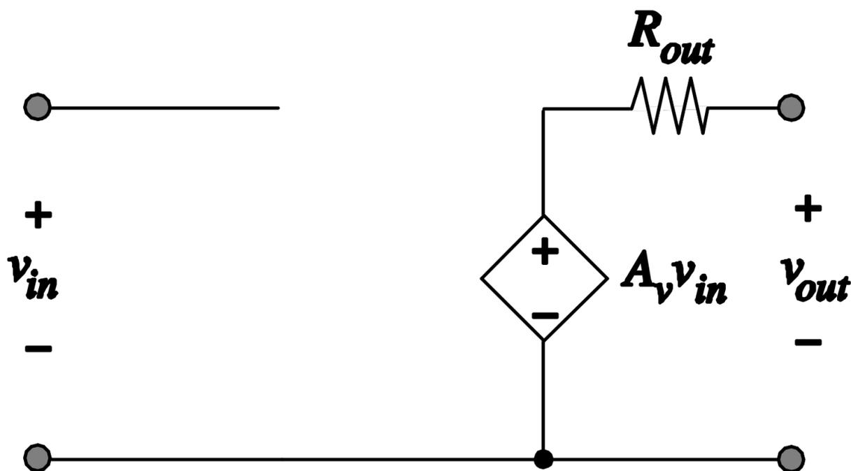
Figure 2.26.: Equivalent voltage amplifier-based model for the common-source amplifier circuit Figure 2.25.
