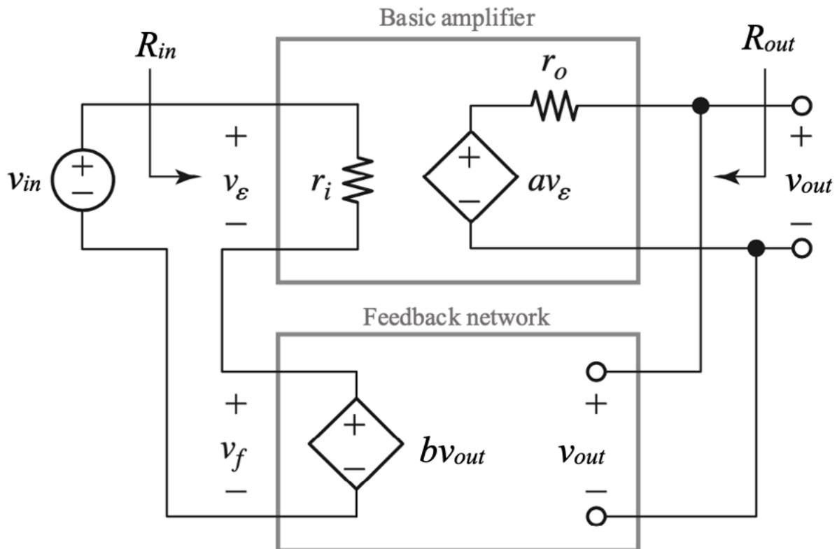
Figure 7.10.: The ideal series-shunt configuration or voltage amplifier (Franco 2015)
