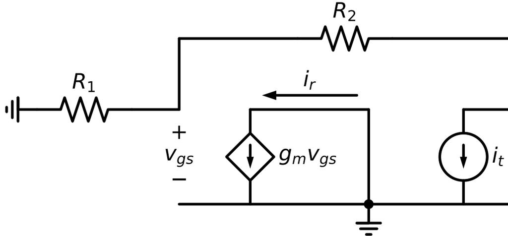
Figure 7.38.: return ratio calculation
