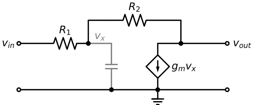
Figure 7.37.: AC equivalent model of the feedback circuit in Figure 7.36
