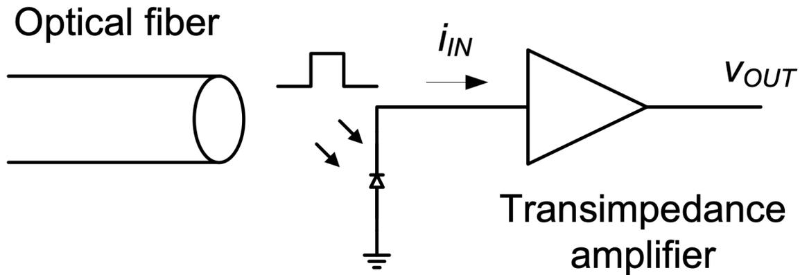
Figure 1.4.: Photodetector circuit for fiber-optic communication.
