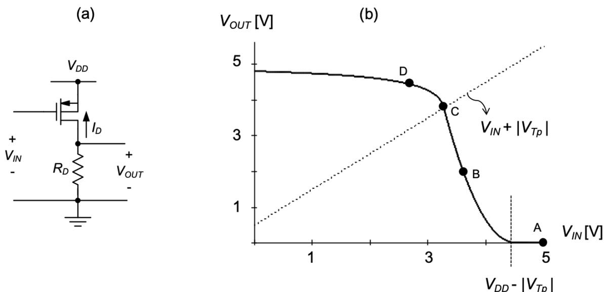
Figure 2.15.: (a) P-channel common-source amplifier schematic. (b) Voltage transfer characteristic for  $V_{DD} = 5$  V,  $R_D = 5$  k $\Omega$ , and  $W/L = 40$ .
