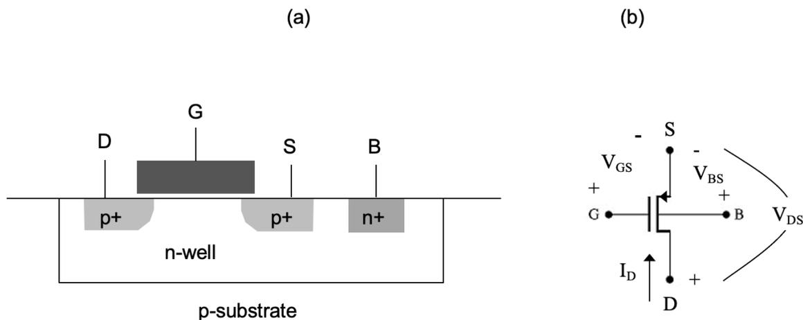
Figure 2.6.: (a) Cross-section of a p-channel MOSFET. (b) Schematic symbol.)
