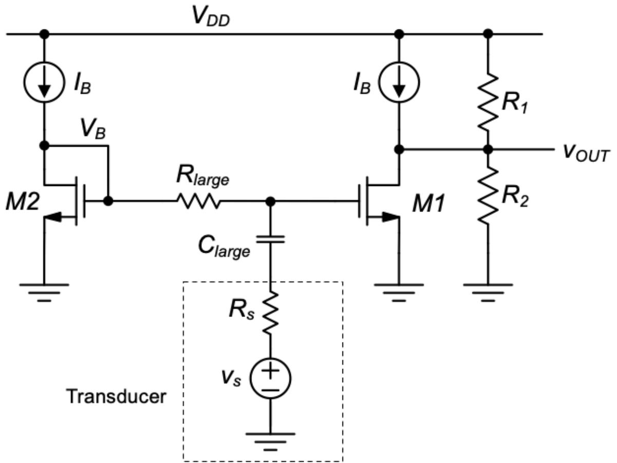
Figure 5.29.: Replica biasing approach using AC coupling.
