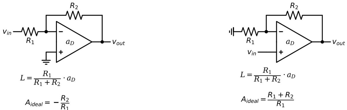
Figure 7.25.: comparison between inverting and non-inverting topology
