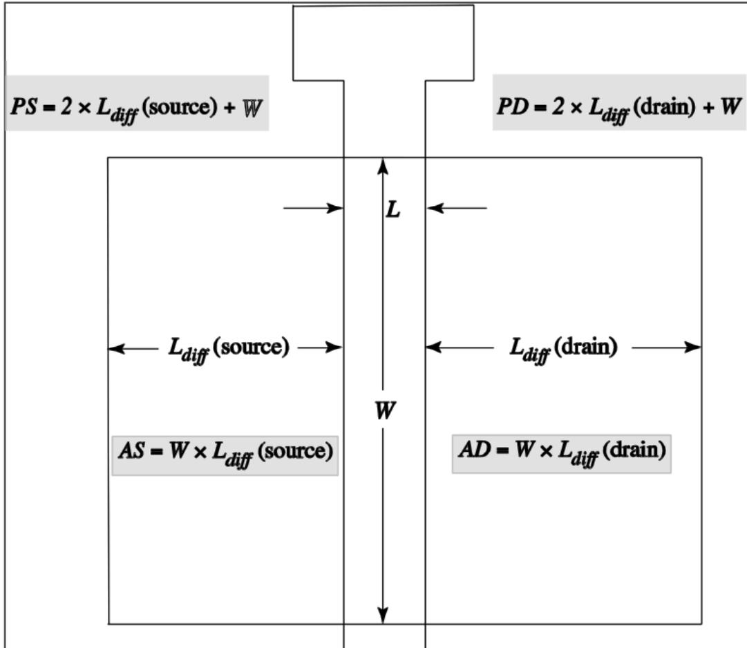
Figure 3.13.: Geometry parameters used for the calculation of junction capacitances.
