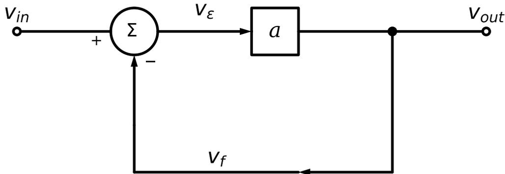
Figure 7.3.: Block diagram of a voltage buffer.
