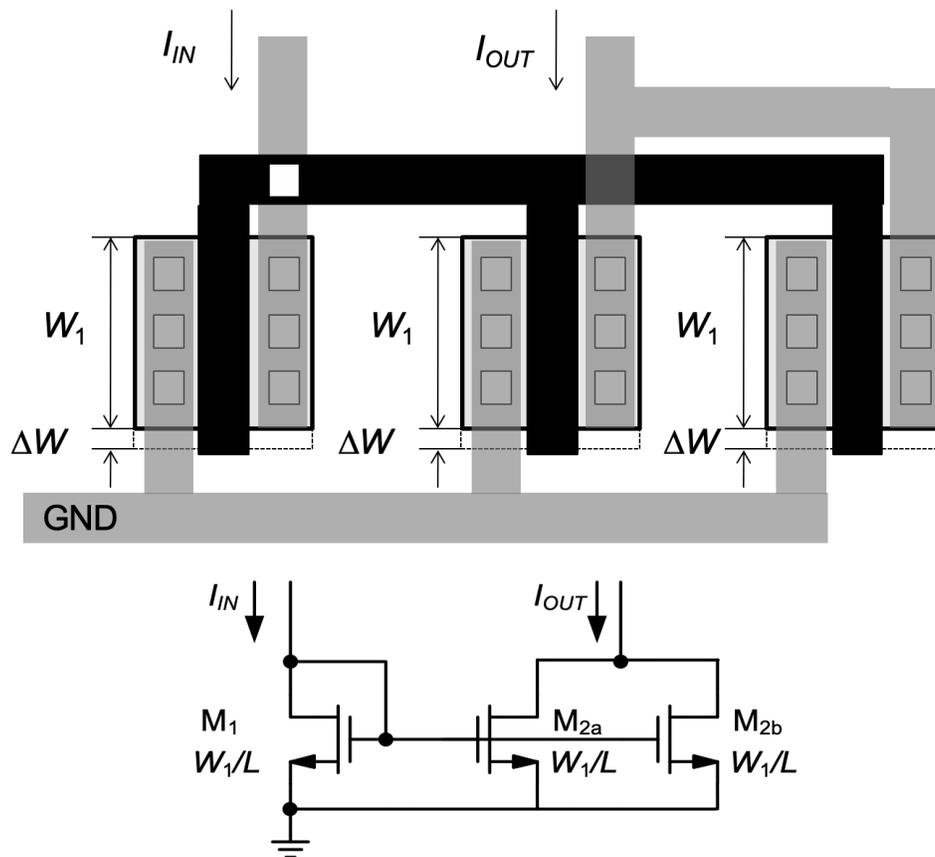
Figure 5.6.: Improved layout of a current mirror with a desired current ratio of two.
