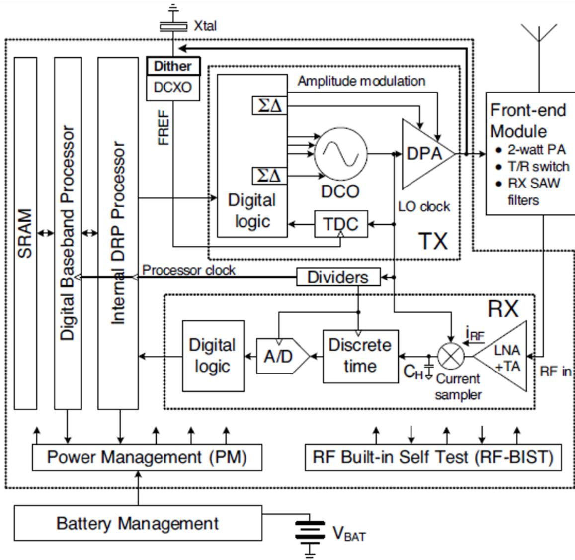
Figure 1.2.: Block diagram of a single-chip radio (Staszewski et al. 2008).
