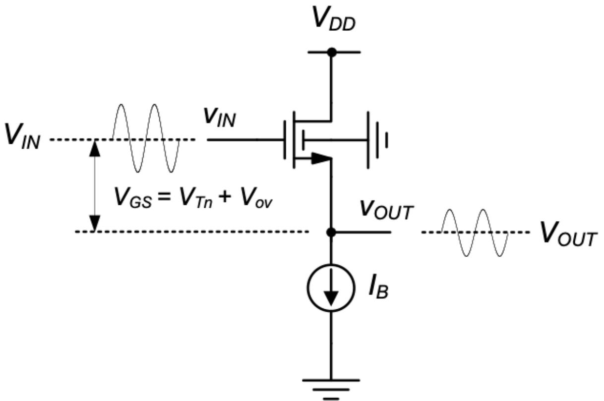
Figure 5.32.: Relationship between the input and output quiescent points in a common-drain stage.
