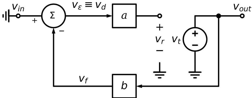
Figure 7.17.: Breaking the Loop.
