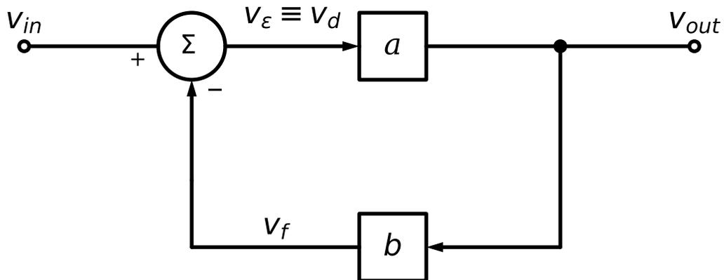
Figure 7.20.: Block diagram of negative feedback system.
