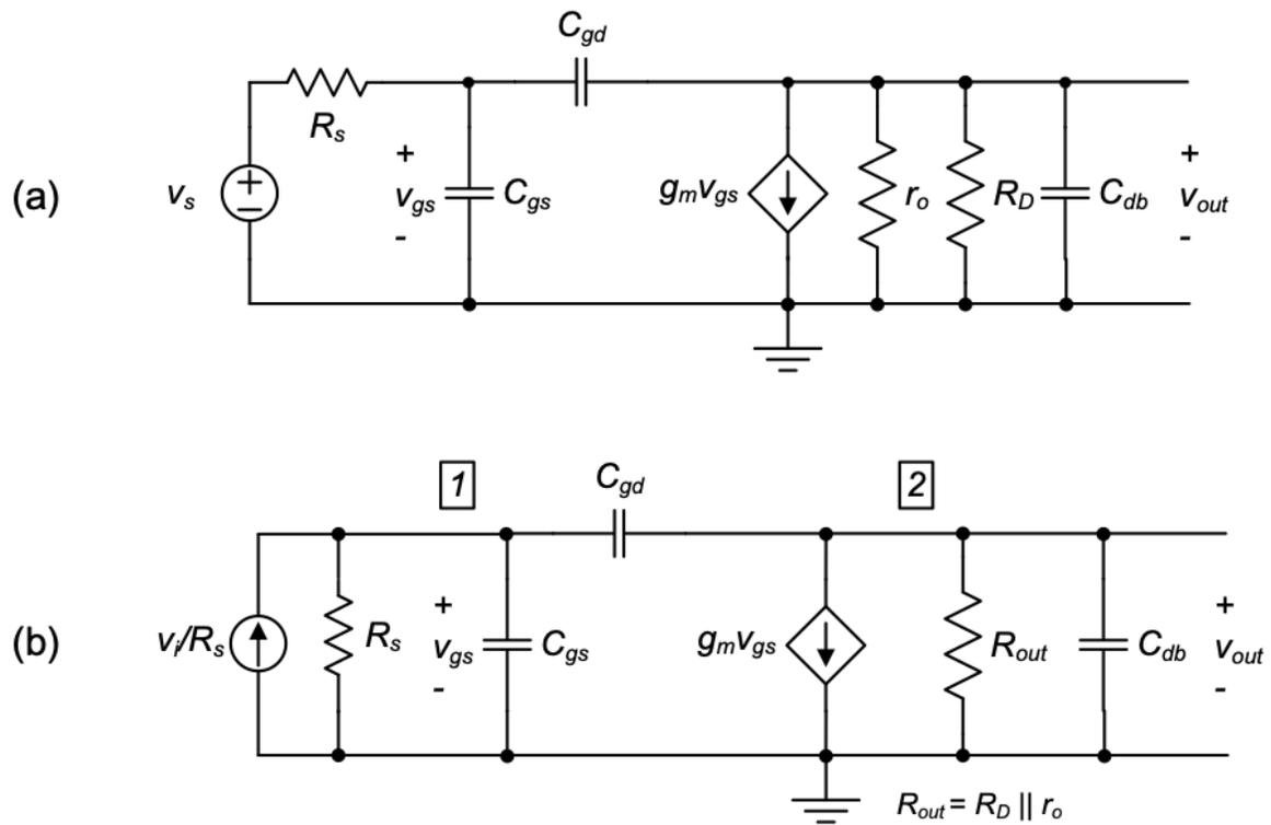
Figure 3.15.: Small-signal model of the common-source amplifier with both intrinsic and extrinsic capacitances included. With (a) Thevenin equivalent input source configuration, and (b) Norton equivalent input source configuration.
