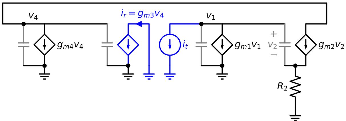
Figure 7.45.: Computing the return ratio for the constant- $g_m$  bias circuit
