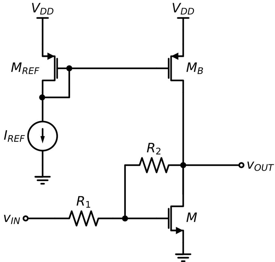
Figure 7.36.: Common source with current-source biasing
