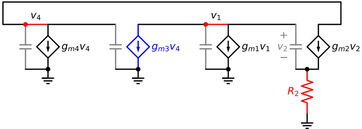
Figure 7.44.: Small signal equivalent model for the constant- $g_m$  bias circuit, (a) red: circuit features that make  $s_t$  insertion not possible, (b) blue: best place for  $s_t$  insertion
