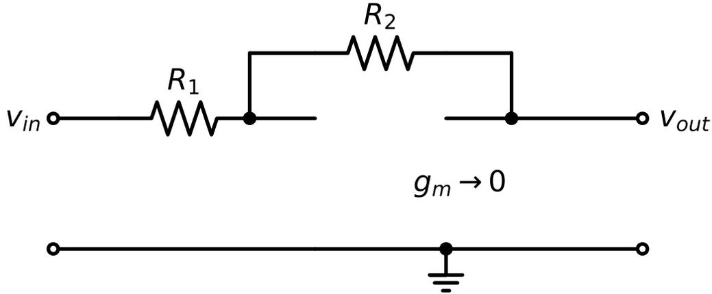
Figure 7.40.: Direct feedthrough calculation
