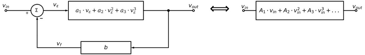
Figure 7.8.: Effect of negative feedback on non-linearity
