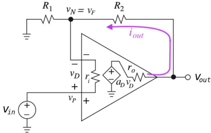
Figure 7.16.: Non inverting op amp amplifier (Franco 2015).
