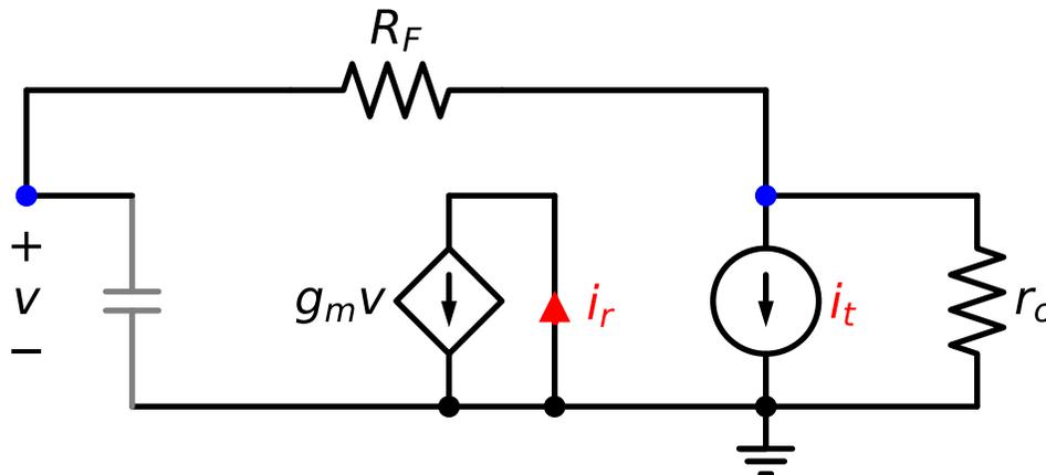
Figure 7.65.: Small signal model to find the return ratio for  $g_m$
