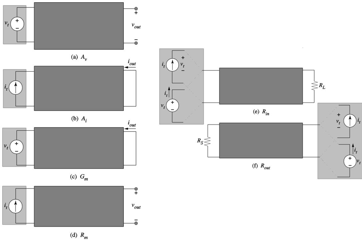
Figure 1.14.: Method to calculate two-port amplifier model parameters: (a) voltage gain  $A_v$ , (b) current gain  $A_i$ , (c) transconductance  $G_m$ , (d) transresistance  $R_m$ , (e) input resistance  $R_{in}$ , and (f) output resistance  $R_{out}$ .
