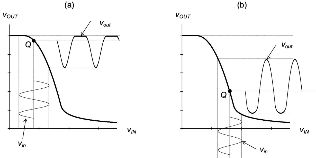
Figure 2.12.: Examples of signal clipping and distortion. (a) Output waveform is clipped due to supply voltage limit. (b) Output waveform drives the MOSFET into the triode region.
