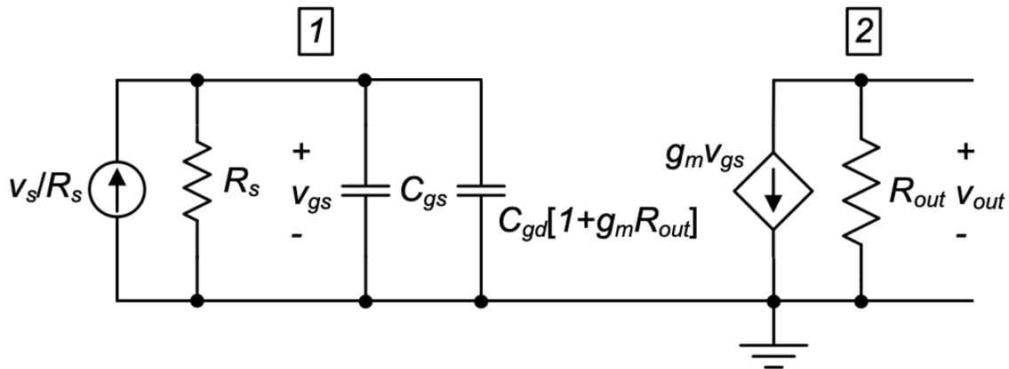
Figure 3.20.: Small-signal model of the common-source amplifier after applying the Miller approximation.
