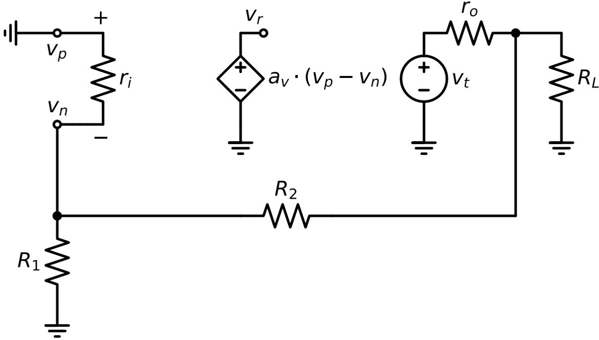
Figure 7.51.:  $T(\text{with input port shorted})$  for non inverting configuration
